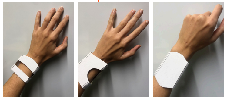
Cardboard prototypes used to test the wearable's comfort on the wrist.
