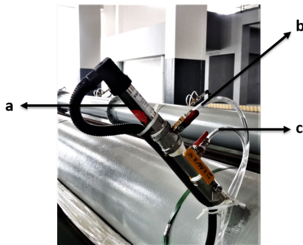
Figure 3.7: Pressure sensor set with total pressure sensor (a), differential pressure sensor impulse tube (b), venting tube (c)
