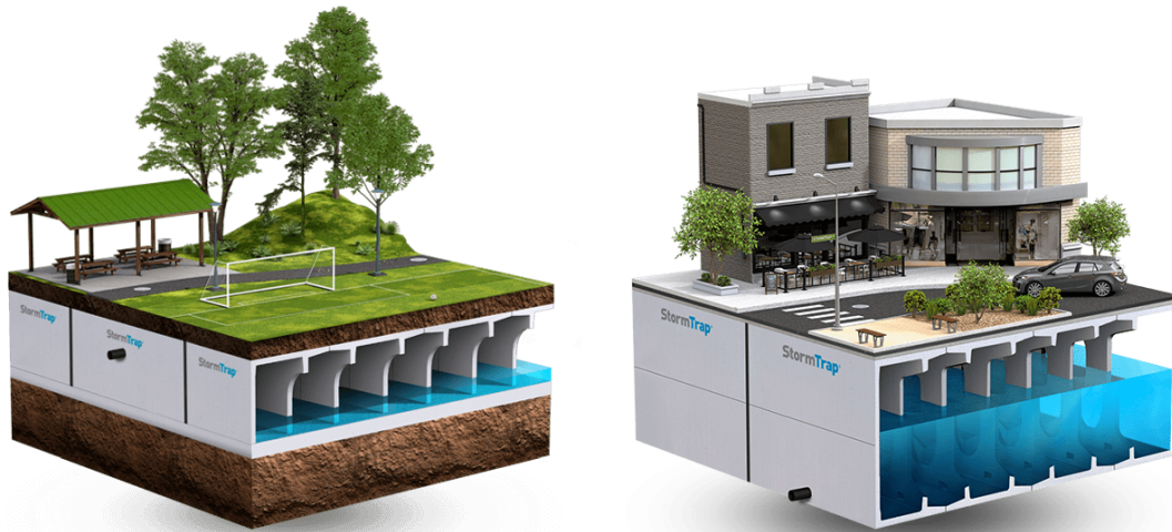
Figure 6.3: Stormtrap underground stormwater basin (Stormtrap, 2016).
