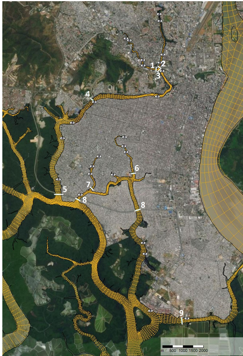
Figure 5.6: Observation points and cross-sections in the Delft3D-FM model
