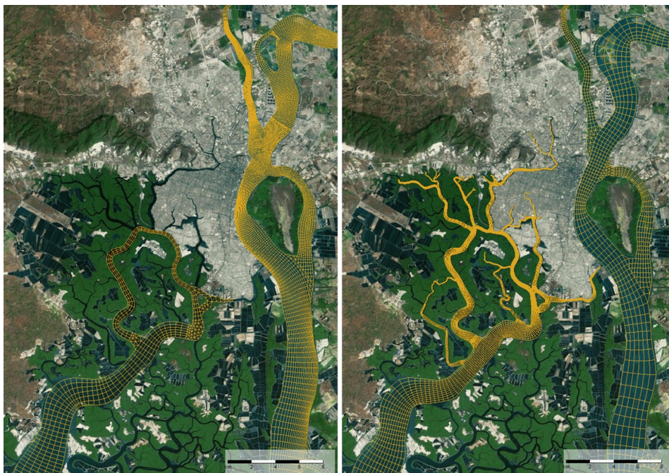
Figure 5.1: Unstructured grids of the sea branches and Guayas river. On the left, the original model. On the right, the adapted model
