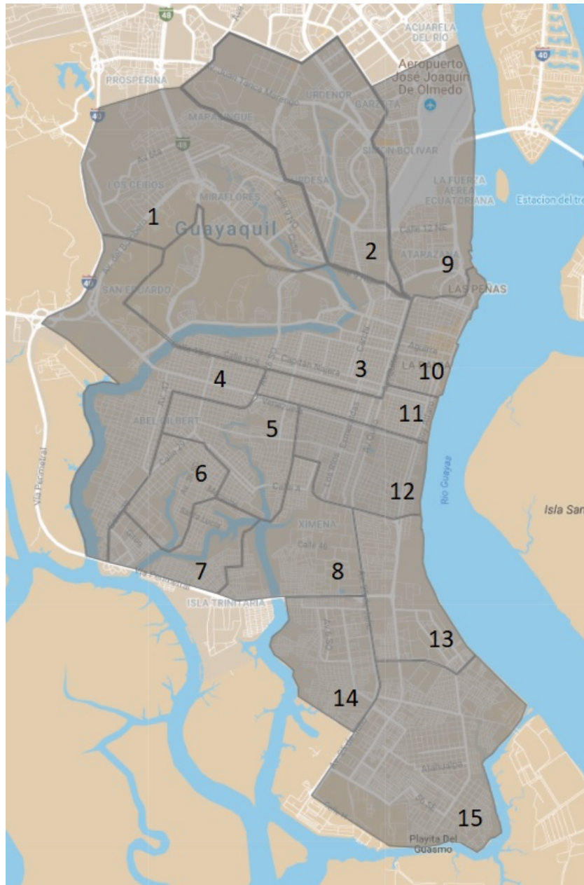
Figure 4.5: Division of the city into catchment areas, based on altitude and stormwater pipe maps (Google, ndb)
