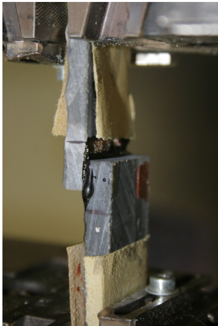
166 167 Figure 2. Flint lap shear sample in test apparatus clamps. Sandpaper was placed between clamps and flint to ensure they would 168 not slip. This photo was taken during the test, and displacement can be witnessed by the distance the ends of the flint have moved 169 from the horizontal black lines.
