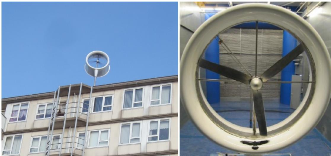
Figure 3.3: DonQi Windmill operating on a rooftop (left) and DonQi with linearised blades in TU Delft Open Jet Facilities (right)
