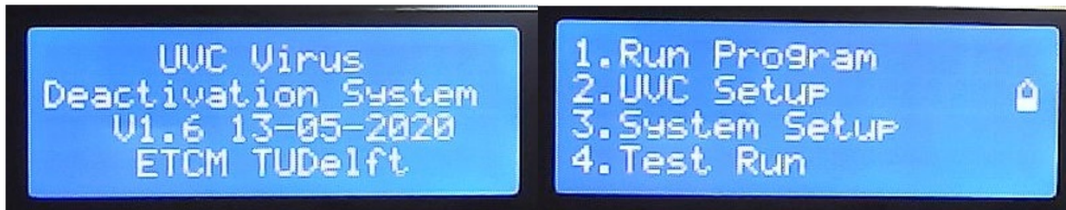
Figure 2.16: Left: Startup screen; Right: Main menu, the lock sign at right of the screen means the kill switch is open, LEDs will not glow
