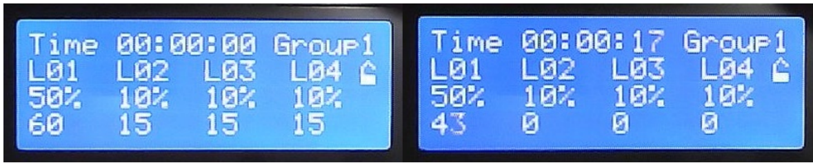
Figure 2.19: Left screen is entering experiment running mode; Right screen is starting the experiment for 17 seconds.
