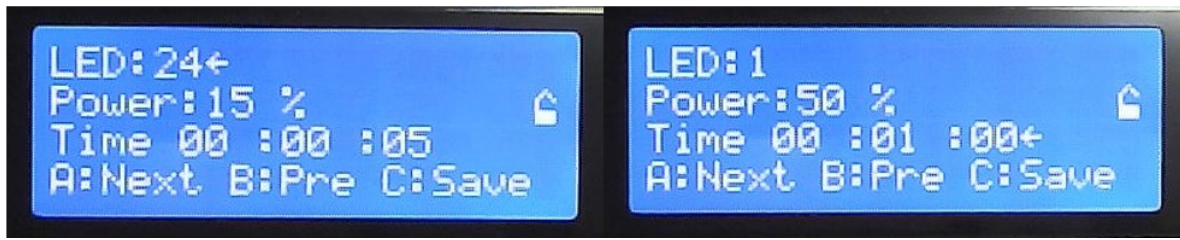
Figure 2.18: Left screen is experiment setup; Right screen is setting LED1 to be 50% power and 1 minute time
