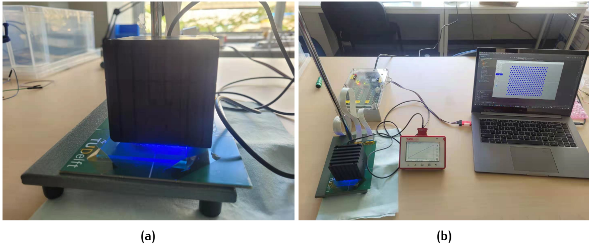
Figure 3.22: (a) Thorlabs S142C placed on the center of the matrix. (b) The overall measurement setup.
