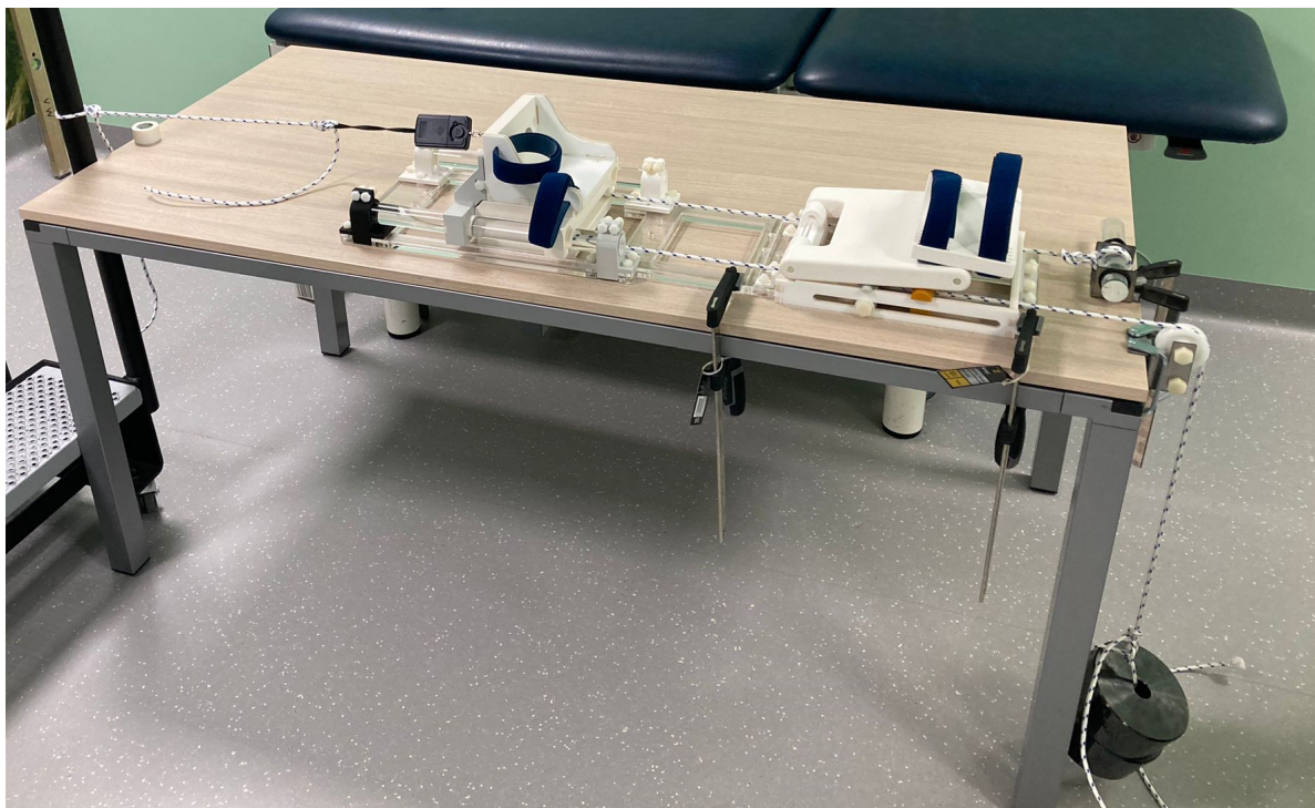
Figure 8.3: The experimental set-up for evaluating the functionality and performance of the load application at the footplate.
