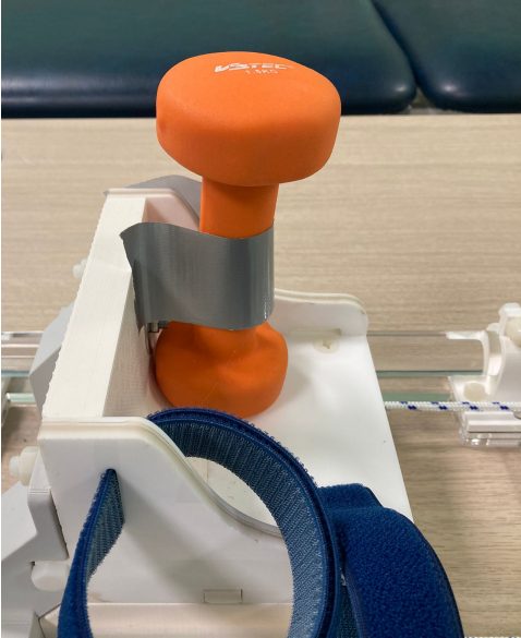
Figure 8.7: Footplate with 1.5 kg the force mimicking the vertical force of the foot resting on the footplate.
