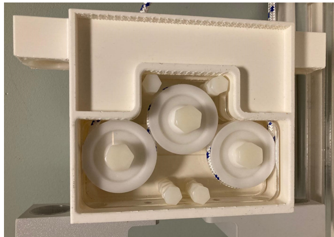
Figure 10.3: Pulleyblock and footplate with a tight fit.
