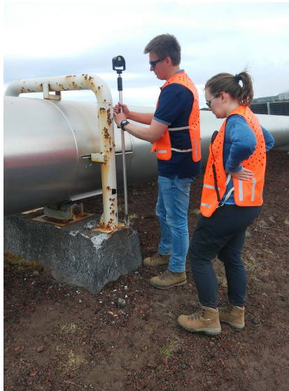
Figure 1.1: Portable prism used to measure the area of the Krafla power plant.
