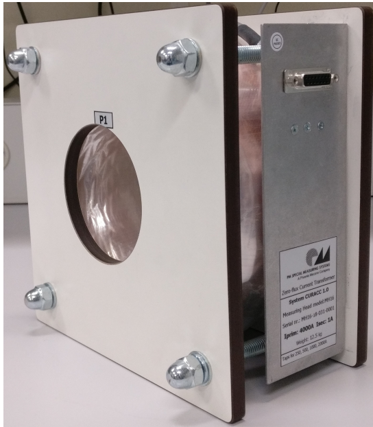
Figure 4.15: Zero-flux current sensor rated for 4000 A
