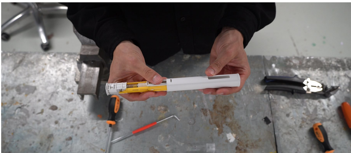
Figure 28 - Photo of the destructive disassembly process and some of the required tools.
