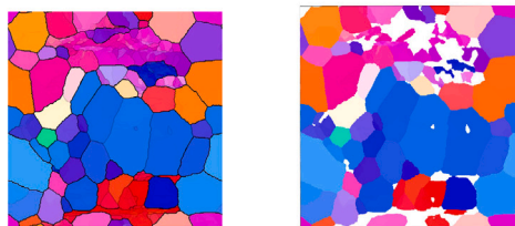
(c) CR (sample 2) - 20 s at 800 °C - f_{rx} = 0.90 .
