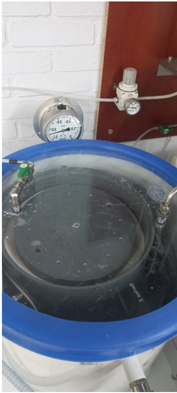
(a) Plate onto the sample to decrease heaving
