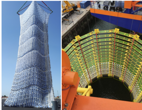
Figure 1.7: The HSD system on the left and the newly developed AdBm-NAS system showing the resonators in the array.(Tsouvalas, 2020). The casings that enclose the pile
