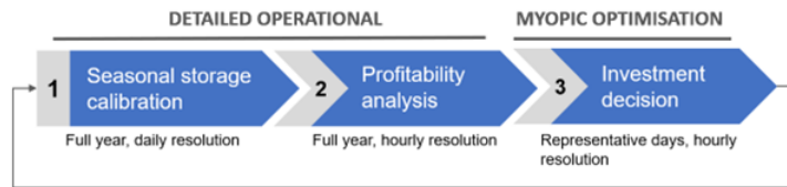
Figure 2.2: Conceptualisation of MODO: three stages with differing temporal settings and input data
