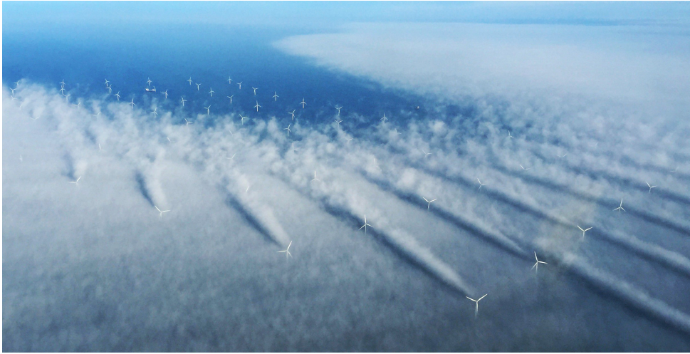
Figure 1.5: Foggy conditions at the Horns Rev 2 offshore wind farm off the coast of Denmark visualize the wake effect. Photo by Bel Air aviation - helicopter services.
