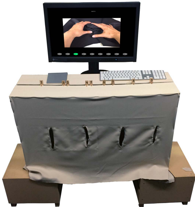
Figure 2. Experimental setup. In the wooden box, behind the curtain, nine fabrics hung indicated by the nine labels. Observers could feel the fabrics through the holes. Behind the box, a computer screen displayed the visual stimuli.
