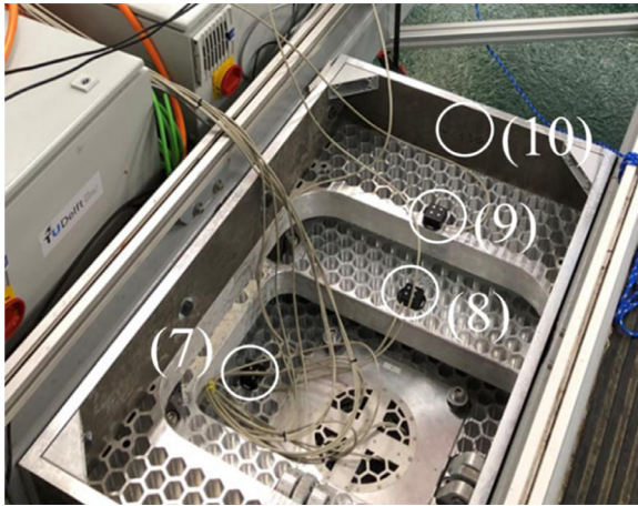
Fig. 11. Test setup mounted to the carriage, showing the accelerometers on the bottom table (7), the middle table (8) and the top table (9). The bottom table moves in x - and y -direction as driven by the actuators. The middle table only moves in y -direction. The top table is fixed to the carriage through an aluminium support frame (10).
