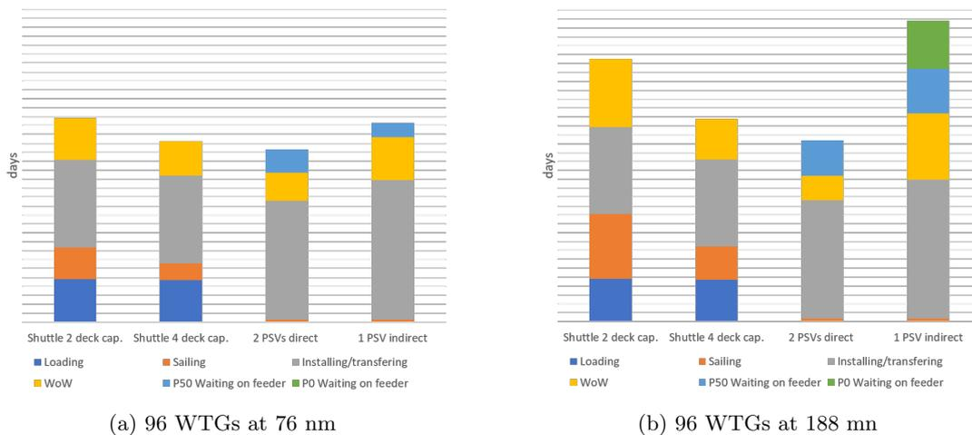
Figure 5.16: Scenario 22, installation vessel activity breakdown
