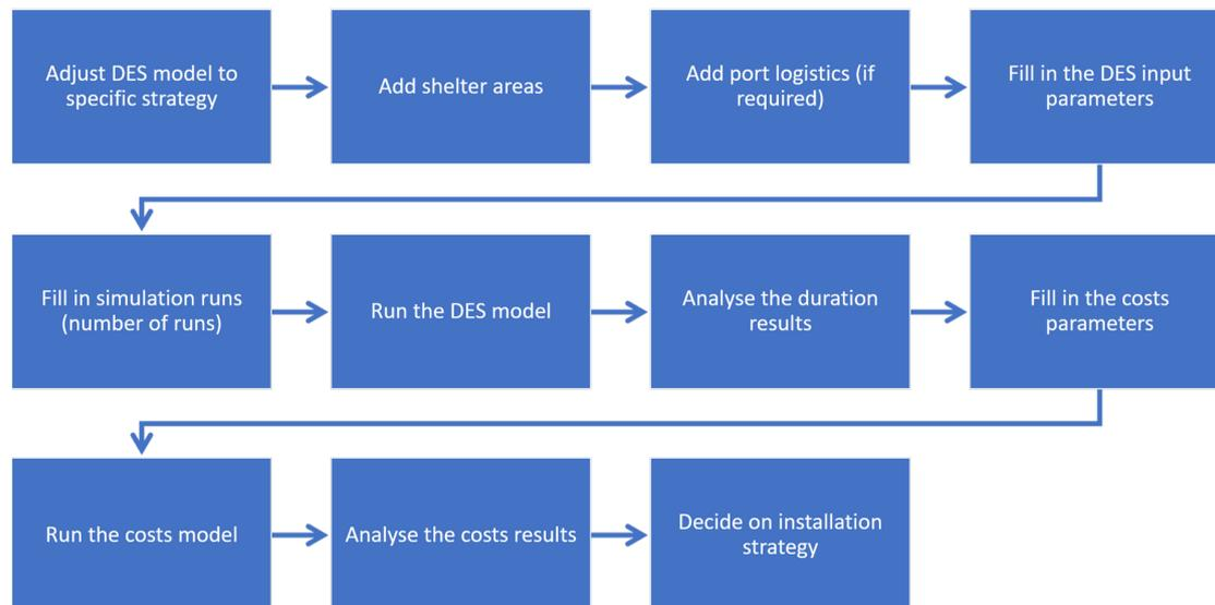
Figure 6.1: Process of how to adapt and run the DES and cost model.
