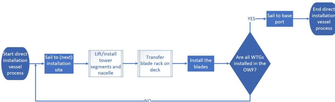
Figure 3.11: Simplified RFD of the installation vessel process for the direct option
