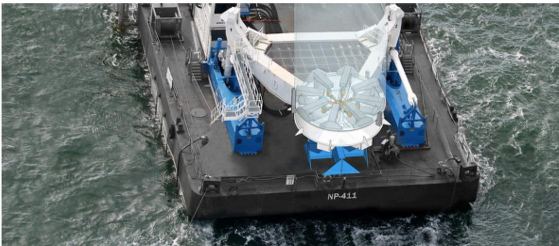
Figure C.2: Barge master motion compensation tool (Bare Master, 2021)
