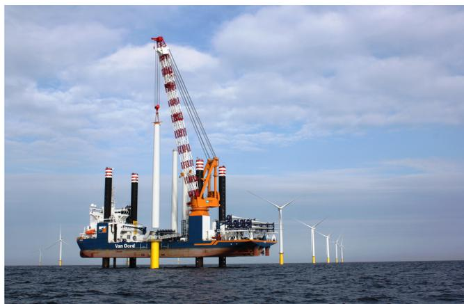
Figure 2.1: The Aeolus installation jack-up vessel of Van Oord installing WTG components
