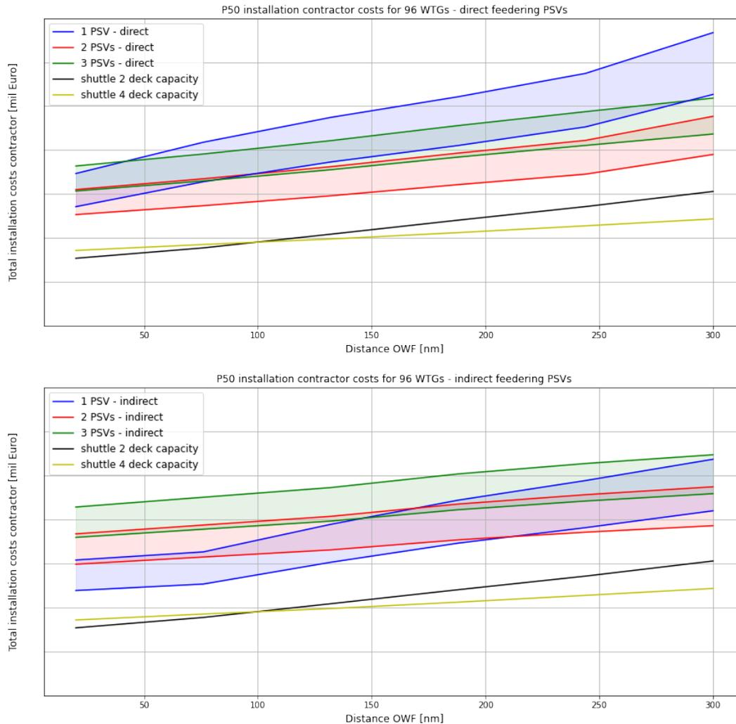
Figure 5.7: P50 contractor cost plot for 96 WTGs with 4 tower segments
