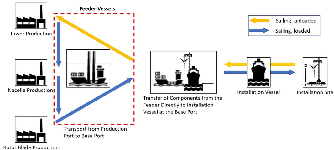
Figure 2.3: The base port feeder method visualised based on Ait Alla et al. (2017)
