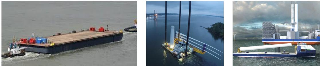
Figure 2.2: (a) An example of a (feeder) barge (Van Loon Maritime Services B.V., 2020), (b) An example of a jack-up feeder (Rochas, 2018), (c) An example of a DP feeder vessel (Blenkey, 2019)
