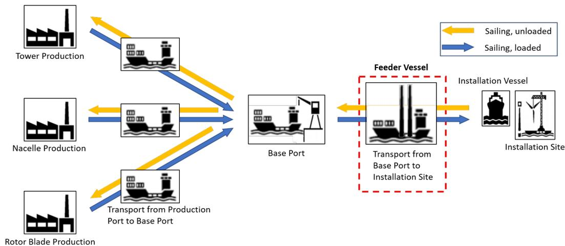
Figure 3.13: The practical feeder-ship method visualised
