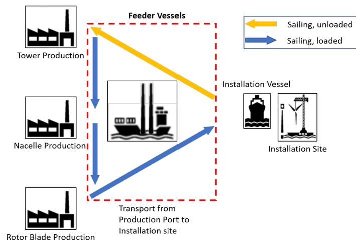
Figure 2.4: The offshore feeder-ship method visualised based on Ait Alla et al. (2017)
