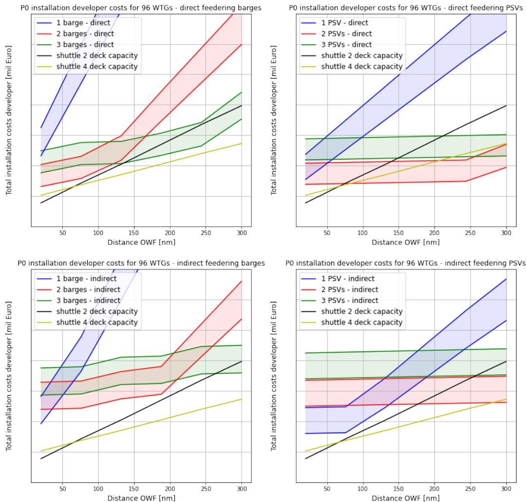
Figure 5.5: P0 developer cost plot for 96 WTGs with 4 tower segments
