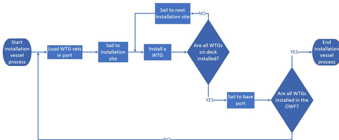
Figure 3.7: Simplified RFD of the installation vessel process for the conventional method
