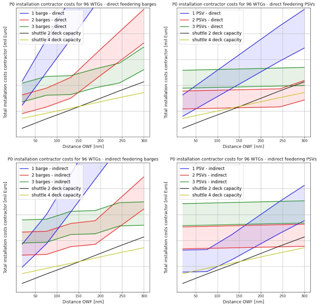
Figure 5.4: P0 contractor cost plot for 96 WTGs with 4 tower segments
