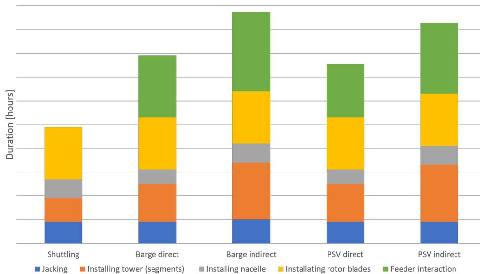
Figure 5.3: P0 single WTG installation and transfer duration breakdown for all strategies (with 4 tower segments)
