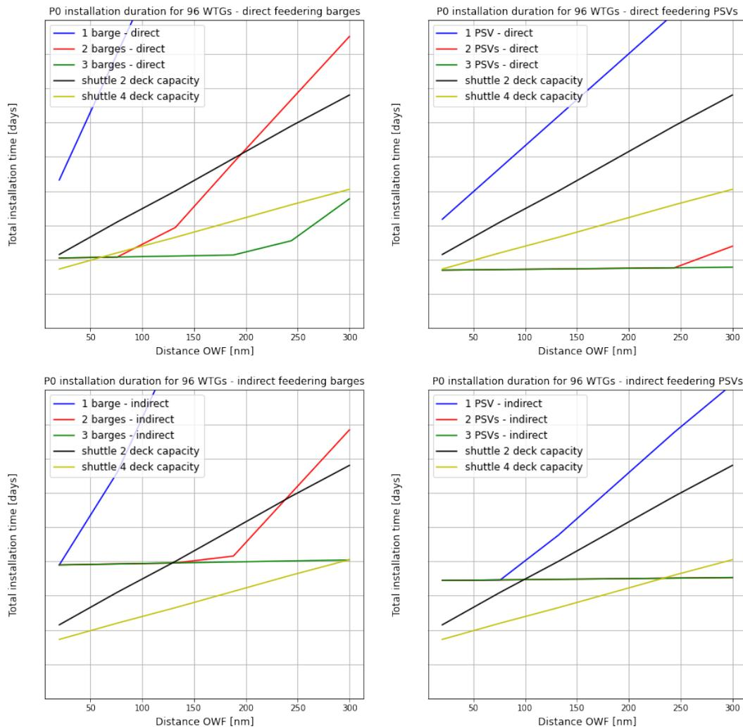
Figure 5.2: P0 duration plot for 96 WTGs with 4 tower segments
