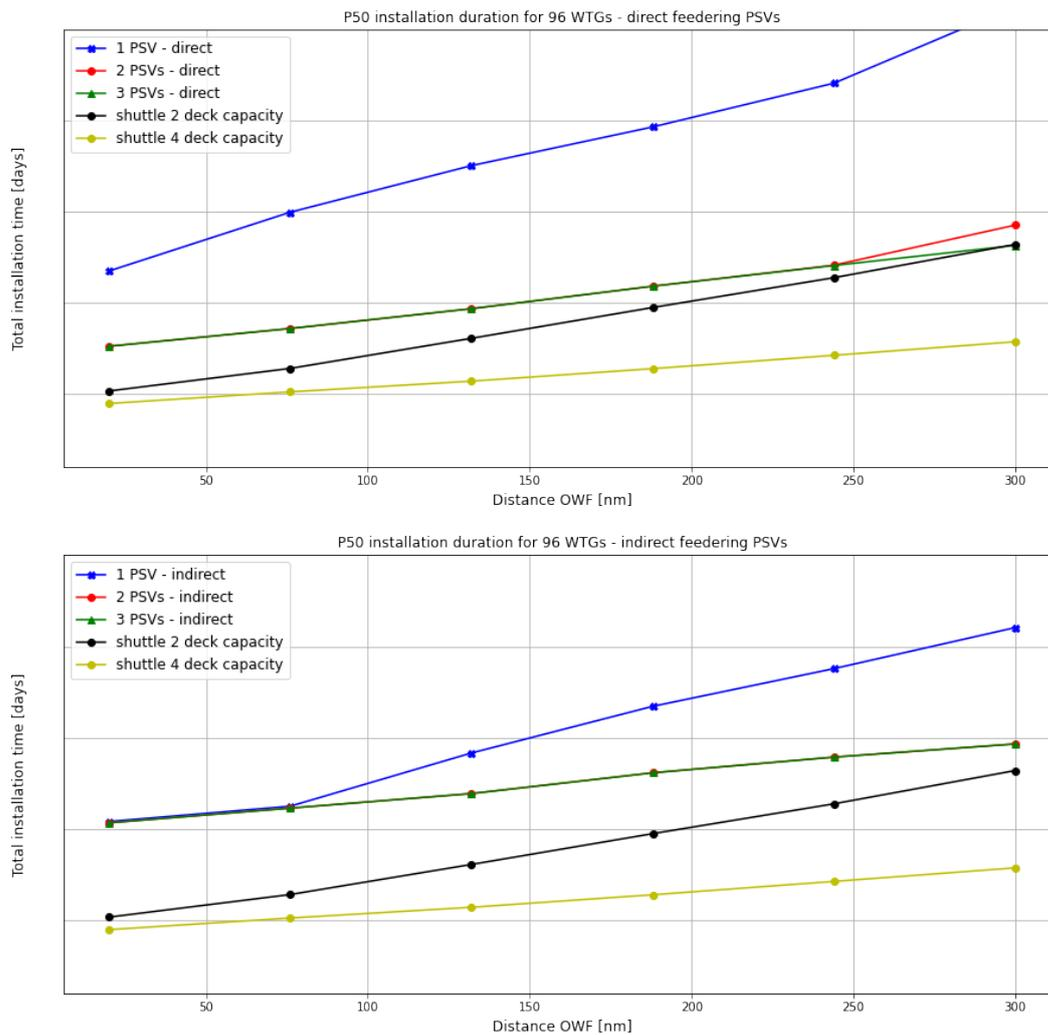
Figure 5.6: P50 duration plot for 96 WTGs with 4 tower segments
