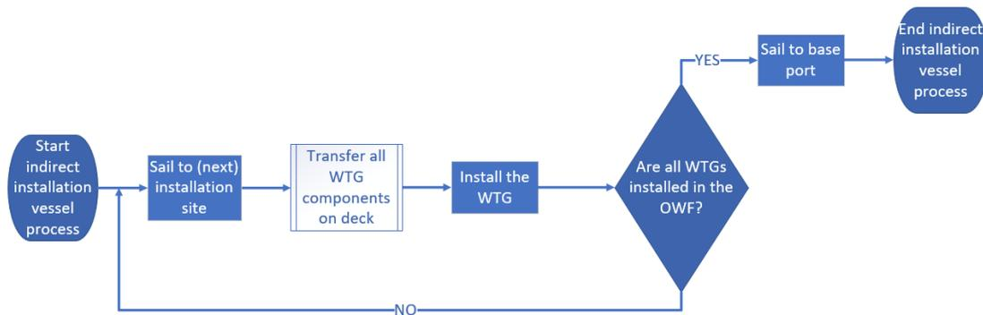
Figure 3.10: Simplified RFD of the installation vessel process for the indirect option
