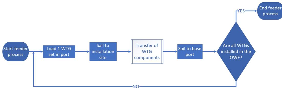
Figure 3.9: Simplified RFD of the feeder vessel process for the feeder method
