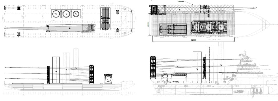
Figure 3.8: (a) Example of a feeder barge layout for a 12 MW WTG (b) Example of a feeder PSV layout for a 12 MW WTG (Van Oord, 2020)
