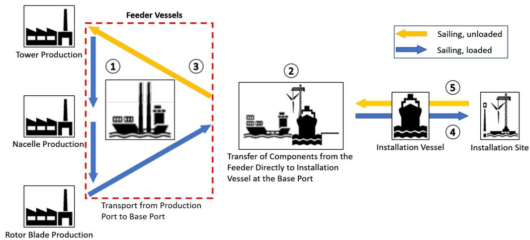
Figure A.2: The base port feeder method steps based on Ait Alla et al. (2017)
