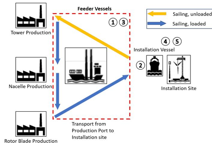
Figure A.3: The offshore feeder-ship method steps based on Ait Alla et al. (2017)
