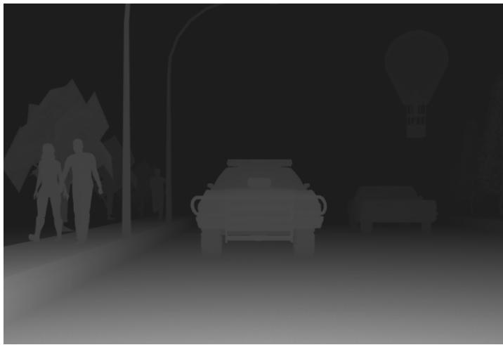
Figure 9: The figure represents a depth image. Objects that are further away from the viewpoint appear with darker color, while objects closer to the viewpoint appear brighter.
