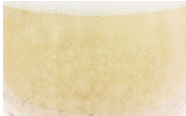
Figure 5. The second processing technique involved liquid shaken cultures of S. commune grown for 7 days from a 7-day culture cultivated from the agar plate as inoculum. The mycelium is then harvested by vacuum filtration and should be stored at -80 degrees or used immediately. The spawn and the liquid culture can be used as inoculum and applied onto composites under aseptic conditions to heal the cracked or broken pieces.
