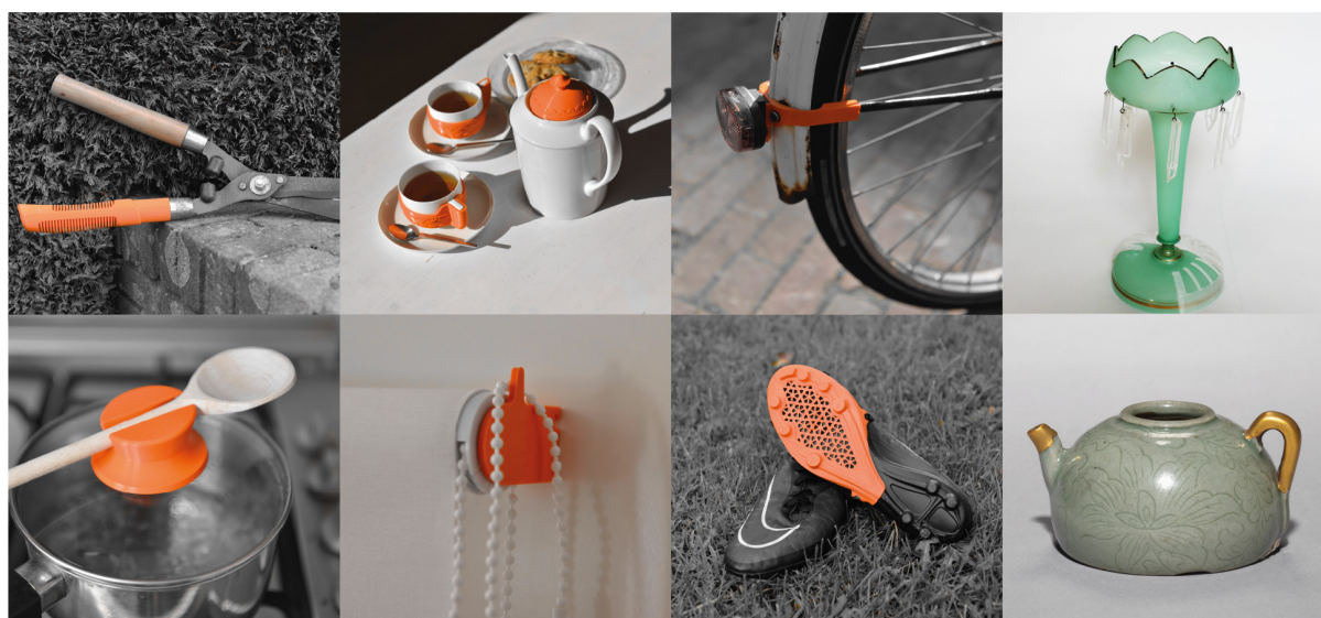
Figure 3. (left) A series of “Value Added Repairs” by Conny Bakker and Marcel den Hollander, exhibited in the Dutch Design Week, showcased how repaired products can be used for longer with the use of 3D printing, without the necessity for expensive stock of spare parts (Blok, 2015); right top) Terzioğlu et. al (2016) explores how they revived an antique 150-year-old Victorian glass lustre through 3D printing technique and mended the piece to bring forth a unique aesthetic; (right bottom) an example of kintsugi repair technique. The movements such as bricolage, DIY practices, and wabi-sabi share the same locus.
