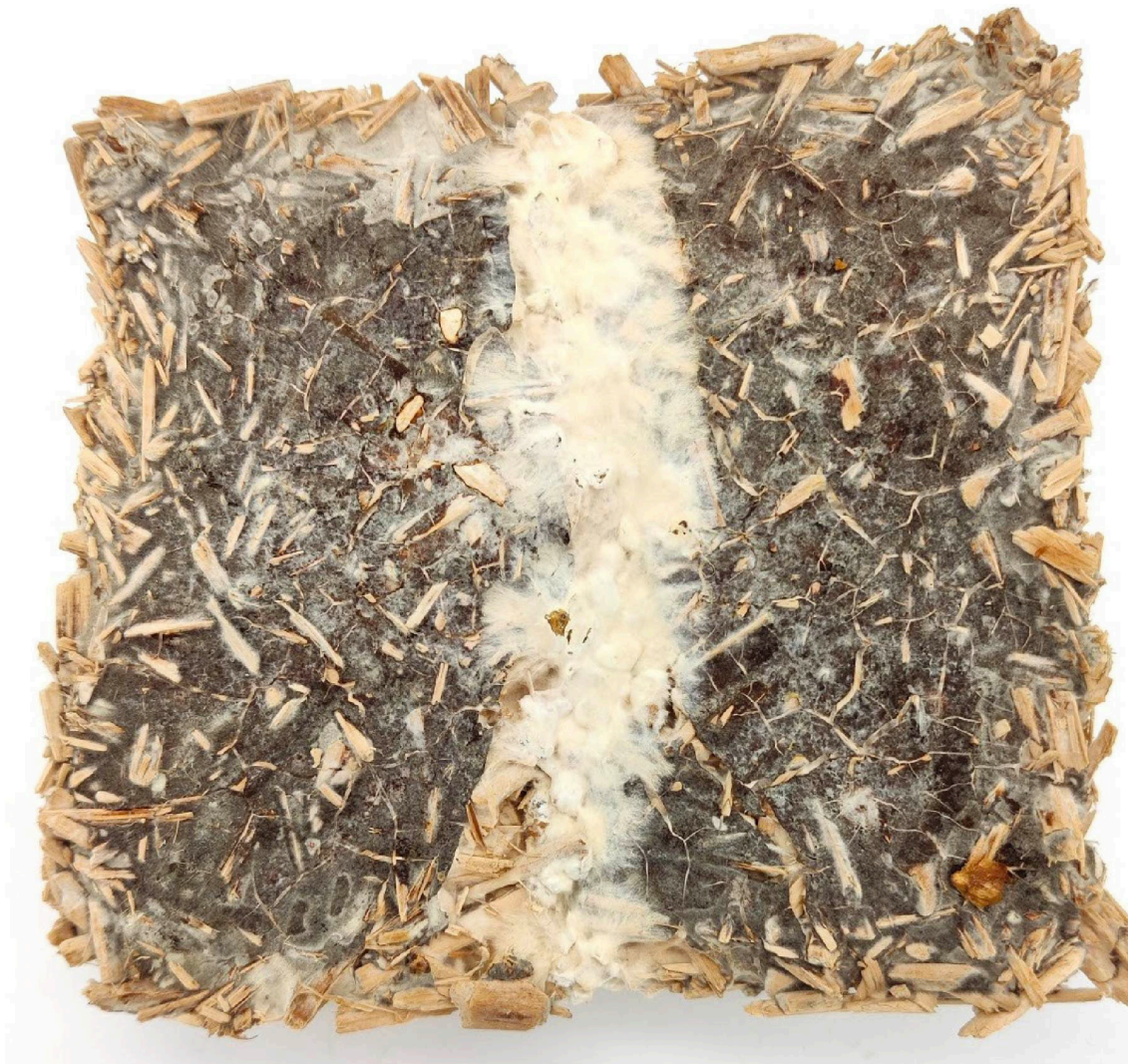
Figure 10. Mended Center trace shows the healing -ability of two non livin broken mycelium composites.
