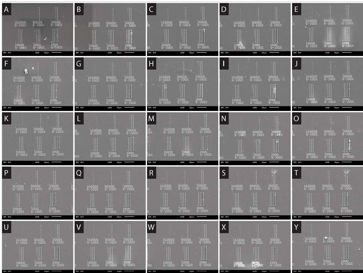
Figure D.52: SEM images of the threshold test performed with the new resist. Each subfigure (A to Y) contains one threshold experiment which was performed every 10 min.
