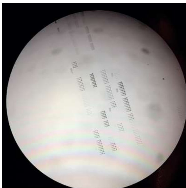
Figure D.55: Resulting mold when printed with the 25x objective onto an oxygen plasma cleaned glass coverslip.
