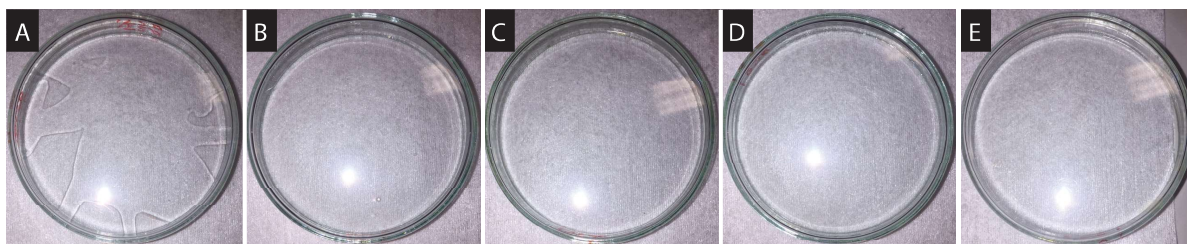
Figure C.50: Results of spin coating the PAA layer at different spin speeds of the second step. A: Image of the spin coated layer of PAA at 250 RPM. B: Image of the spin coated layer of PAA at 500 RPM. C: Image of the spin coated layer of PAA at 750 RPM. D: Image of the spin coated layer of PAA at 1000 RPM. E: Image of the spin coated layer of PAA at 1250 RPM.
