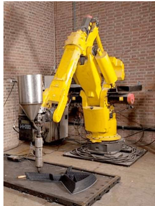
Figure 2-12: a) The Endless chair designed by Dirk van der Kooij. b) The robotic setup used for fabrication (Source: https://www.dirkvanderkooij.com )
