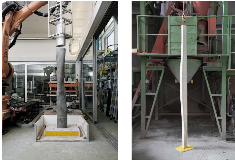
Figure 2-6: a) Column produced using SDC [32] b) Mullion produced for the DFAB House (Source: http://www.dfab.ch/portfolio/smart-dynamic-casting-sdc/ )
