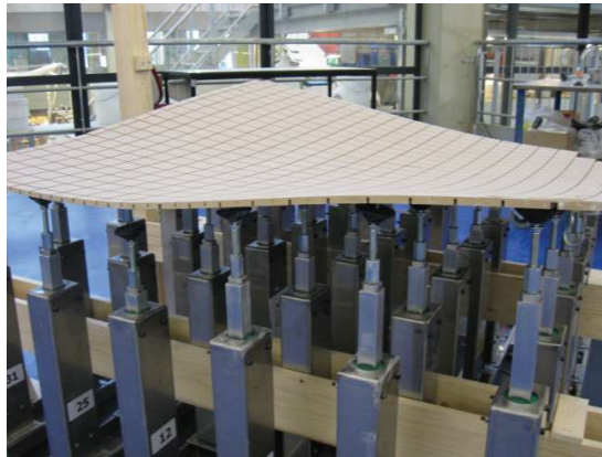
Figure 2-5: a) Flexible mould system from TU Delft [9]. b) Tailorcrete, ETH Zurich, left: wax formwork, right: concrete element [30].
