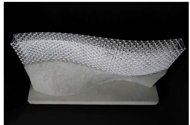
Figure 2-13: Three images showing the spatial extrusion of plastic meshes. a) The robotic arm fabricating a 1:1 scale prototype. b) ABS hardening in mid-air. c) The final mesh structure, half-filled with concrete to create a double curved wall element [38].
