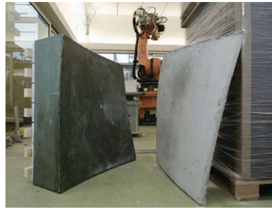
Figure 2-5: a) Flexible mould system from TU Delft [9]. b) Tailorcrete, ETH Zurich, left: wax formwork, right: concrete element [30].
