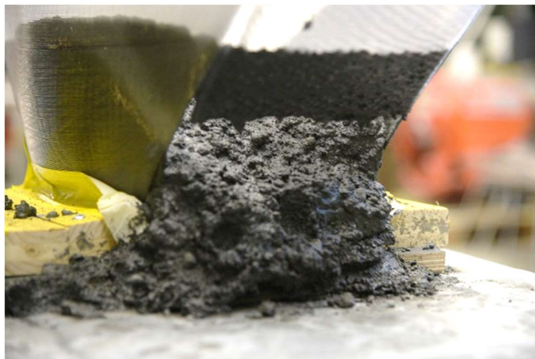
Figure 4-26: Failure of model with 45° overhang.
