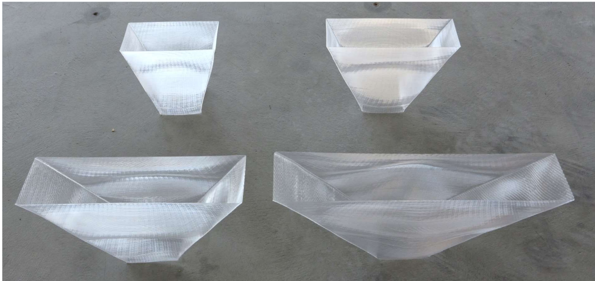
Figure 4-24: 3D printed models to be tested. a) Overhang of 15°. b) Overhang of 25°. c) Overhang of 35°. d) Overhang of 45°.
