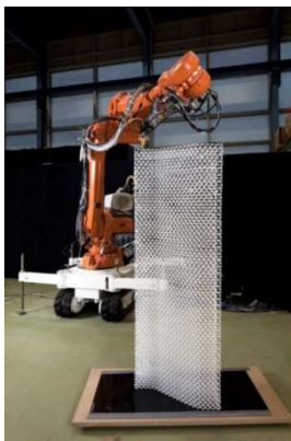
Figure 2-13: Three images showing the spatial extrusion of plastic meshes. a) The robotic arm fabricating a 1:1 scale prototype. b) ABS hardening in mid-air. c) The final mesh structure, half-filled with concrete to create a double curved wall element [38].
