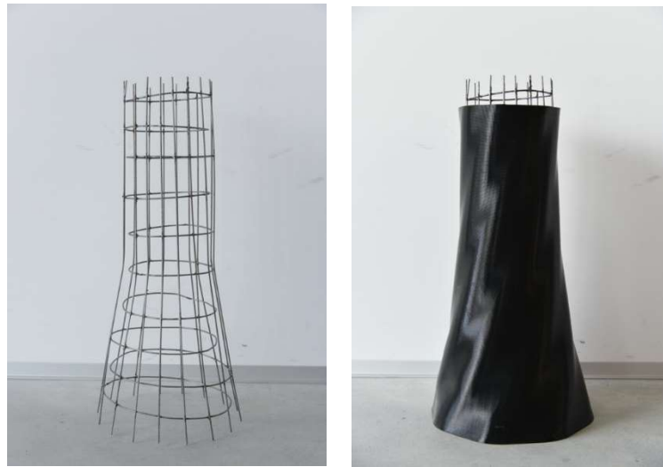
Figure 4-14: Objects used for the experiment, a) Reinforcement cage. b) 3D printed formwork combined with reinforcement cage.
