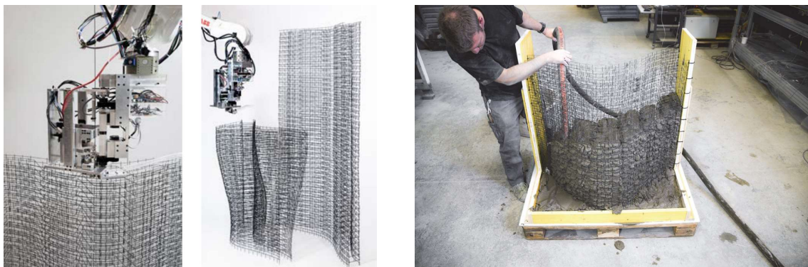
Figure 2-9: a) The Mesh Mould tool head b) Double and single curved metal meshes. c) Filling of a metal mesh with concrete [38].
