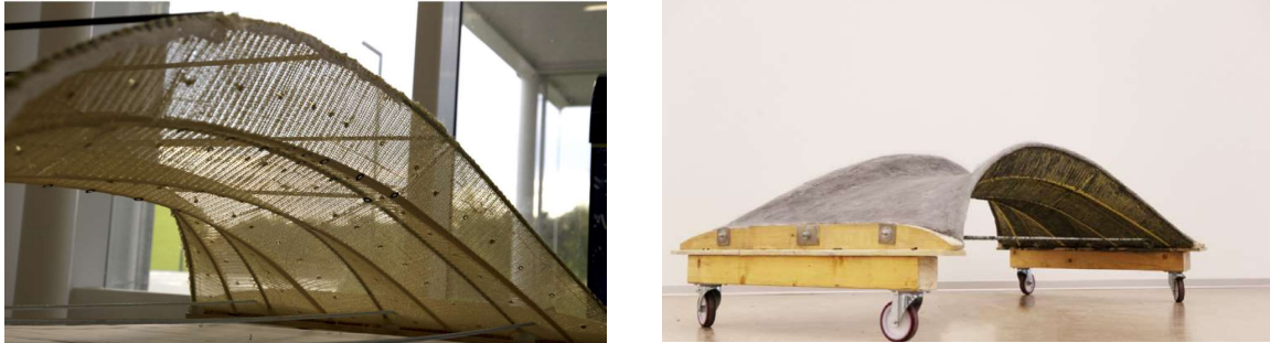
Figure 2-10: a) Knitted formwork underside. b) Finished concrete bridge [39].
