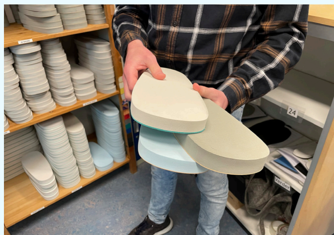
Figure 4.12 - A selection of foam layers with different densities to best accommodate the orthotic specifications of a patient. The foam layers are CNC milled into the 3D modelled design, including the selected elements that are added to the orthotic by the podiatrist.
