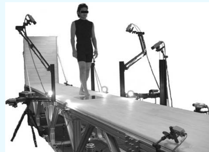
Figure 3.9 - Walkway setup using 12 video cameras to capture the foot (Kimura, Mochimaru and Kanade, 2009).
