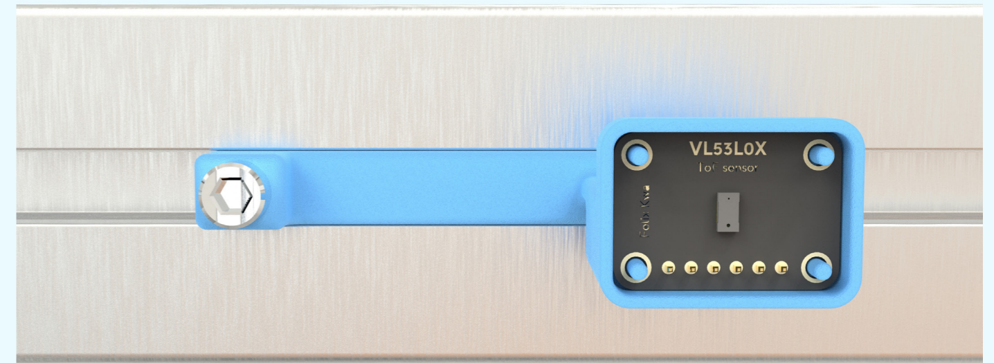
Figure 11.15 - A render of how the ToF sensor is positioned in the mount on the aluminium frame.
