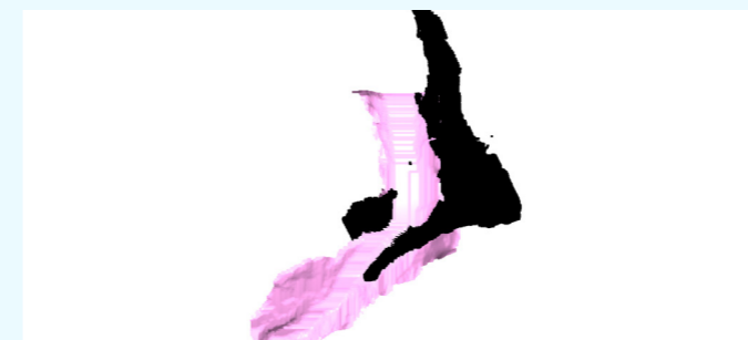
Figure 13.7 - Misalignment of two point clouds after initial alignment and Point-to-Plane ICP.
