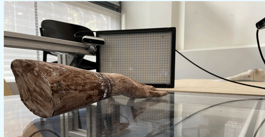
Figure E.6 - The lighting experiment setup.
