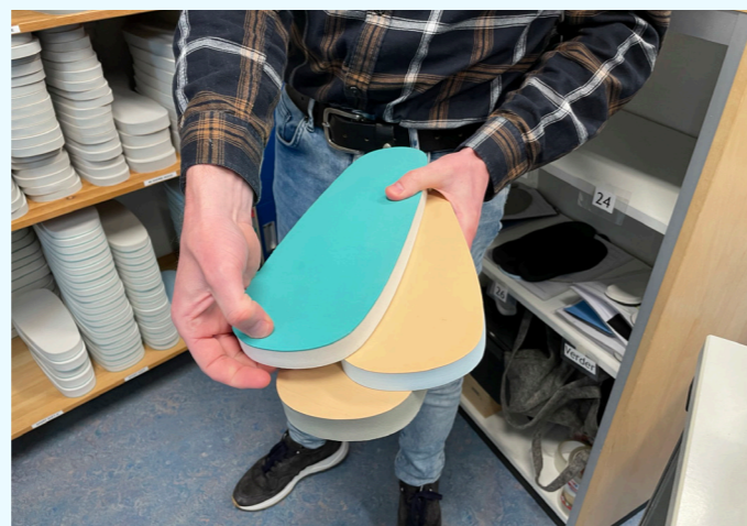
Figure 4.12 - A selection of foam layers with different densities to best accommodate the orthotic specifications of a patient. The foam layers are CNC milled into the 3D modelled design, including the selected elements that are added to the orthotic by the podiatrist.
