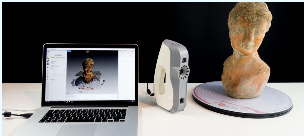
Figure 4.5 - The Artec Eva, a handheld 3D scanner to capture objects (3D Scan Expert, 2017).
