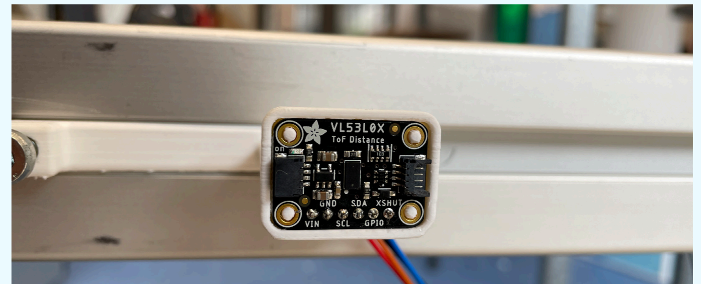
Figure 11.16 - The real life implementation of the ToF sensor in the mount on the aluminium frame.
