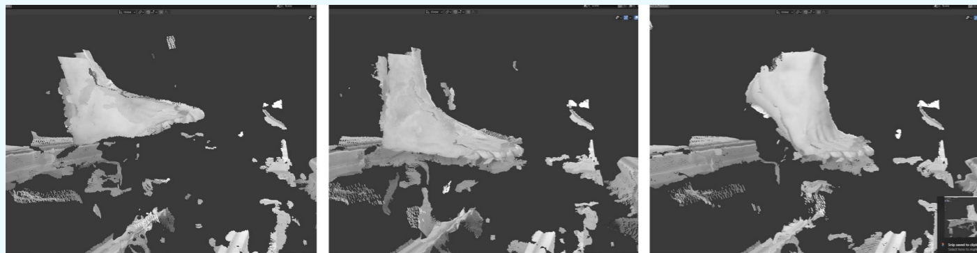
Figure 3.7 - Three frames containing point cloud data of a foot, captured with 4 cameras, observed from an arbitrary point of view in space (Vidmar, 2020).
