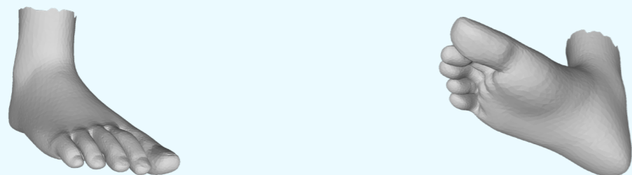
Figure 13.6 - 3D foot model which is used as reference model for nonrigid ICP registration.
