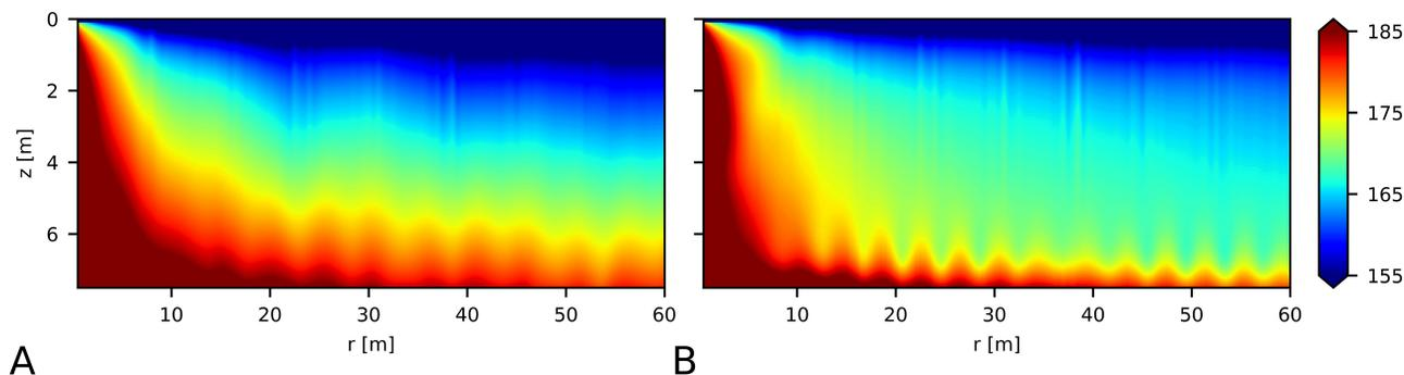
Figure 3: Sound exposure levels in dB integrated over 1 second due to VH (A) and GDP (B) hammering under perfect contact assumption.
