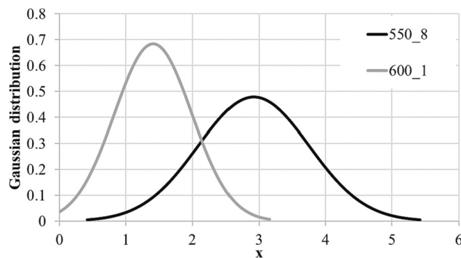
Fig. 7. The gaussian distribution plotted based on the diameter of the \kappa -carbides for the 550_8 and 600_1 samples.
