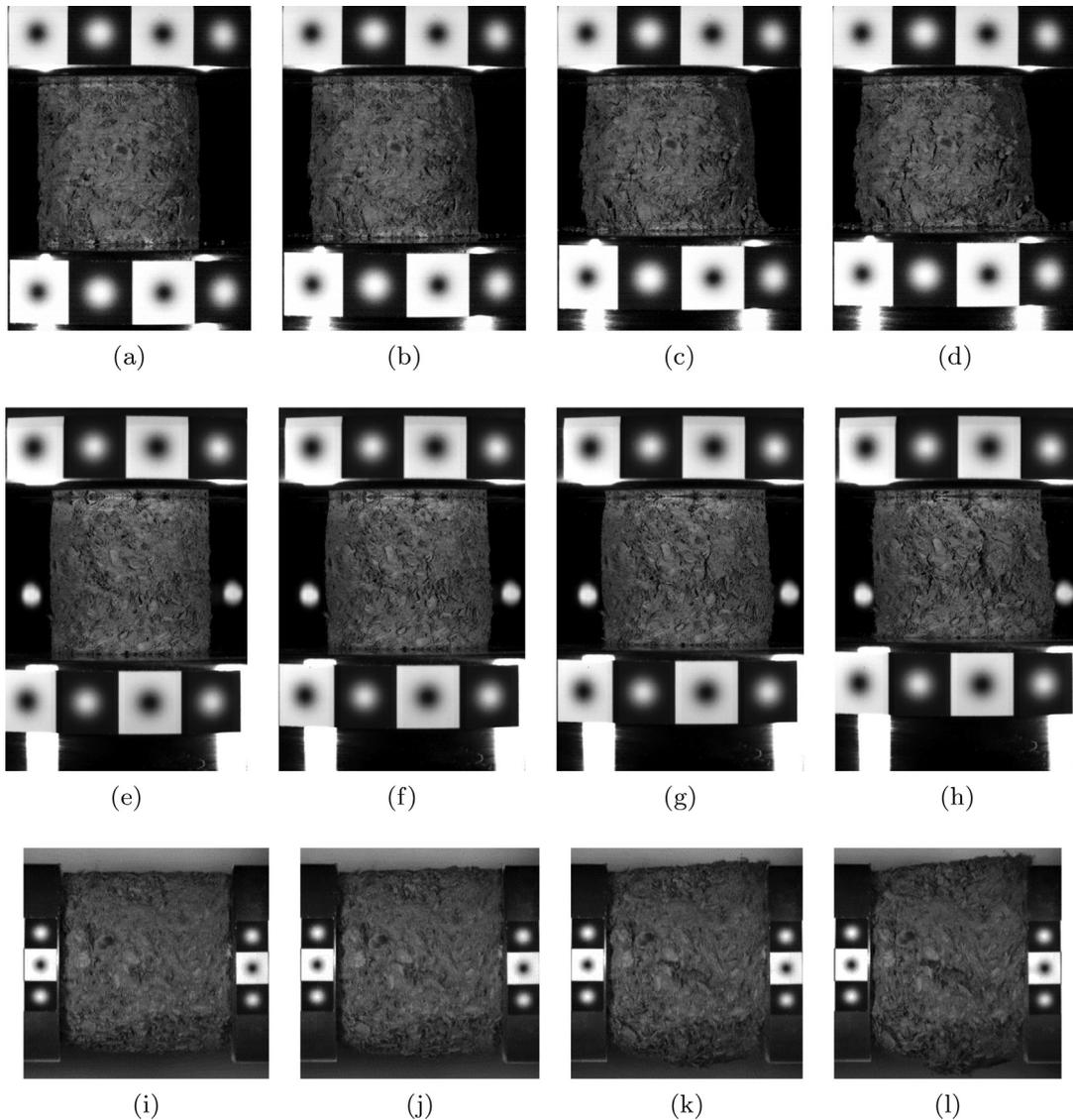
**Fig. 5.** Comparison of typical damage progressions for air dried Type B at first crack appearance and 8%, 12%, 15% strain levels for static test (first row), intermediate strain rate test (second row) and split Hopkinson bar test (third row).
