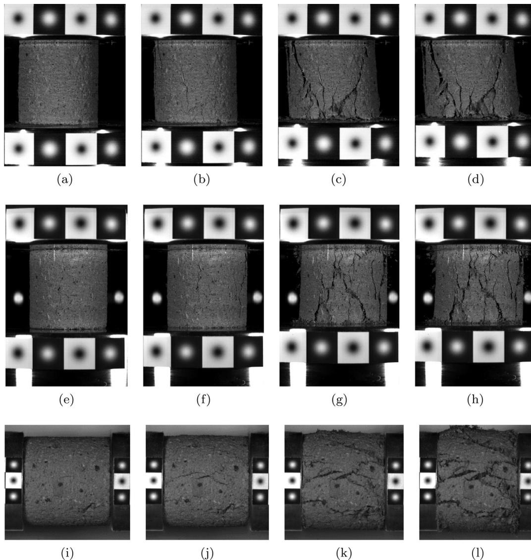
**Fig. 4.** Comparison of typical damage progression for air dried Type A, at first crack appearance and 4%, 8%, 10% strain levels for static test (first row), intermediate strain rate test (second row) and split Hopkinson bar test (third row).
