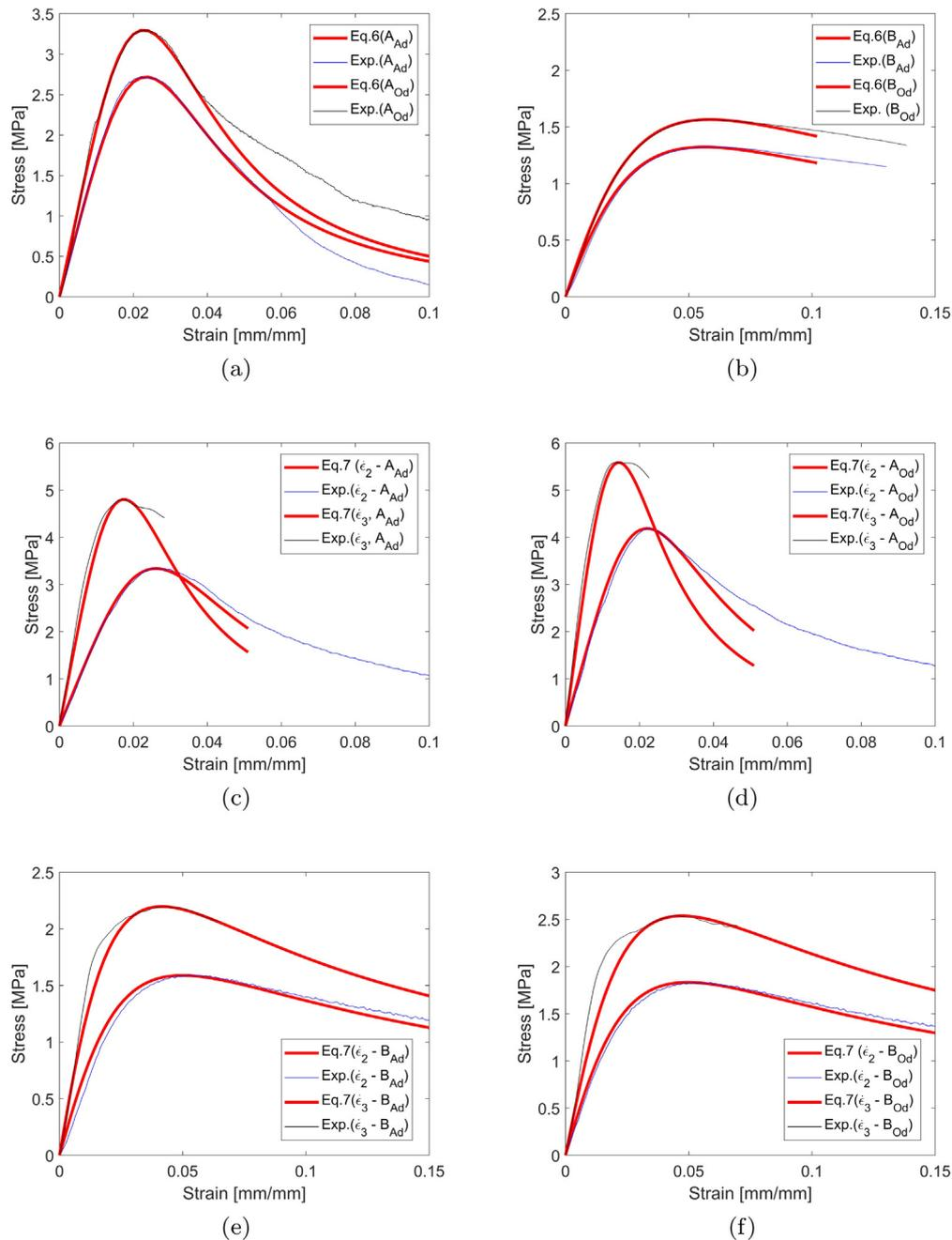
**Fig. 14.** Experimental-analytical comparison in statics for air dried and oven dried Type A (a) and Type B (b) and experimental analytical comparison in dynamics at both strain rates ( $\dot{\epsilon}_2$  and  $\dot{\epsilon}_3$ ) for air dried Type A and Type B (c, d) and oven dried (e, f).
