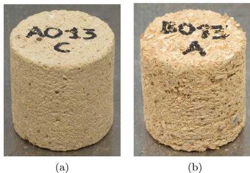
Fig. 1. Example of tested fiber free (a) and fiber reinforced (b) adobe.
