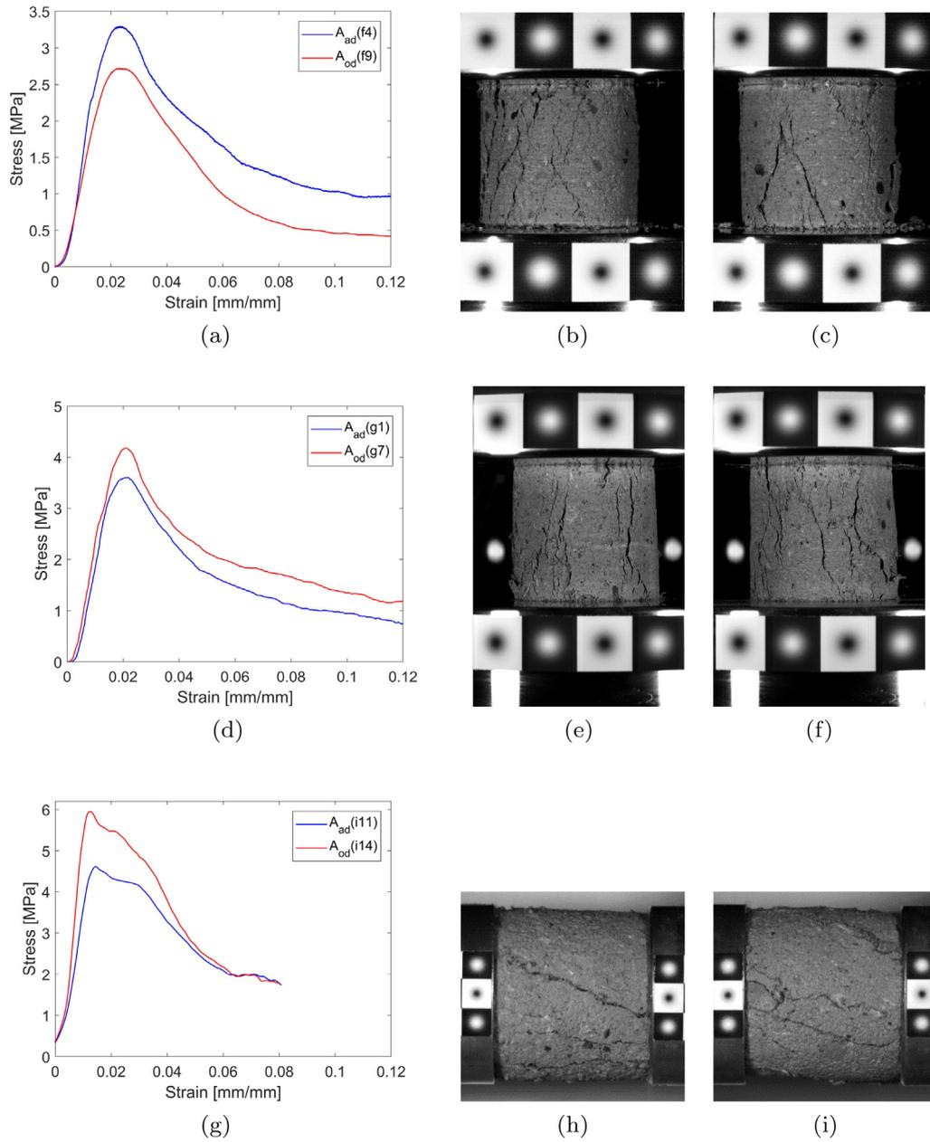
**Fig. 7.** Examples of stress strain plots and corresponding cracking patterns at 50% stress decay for air dried (b, e, h) and oven dried (c, f, i) Type A for static test (first row), intermediate strain rate test (second row) and split Hopkinson bar test (third row).
