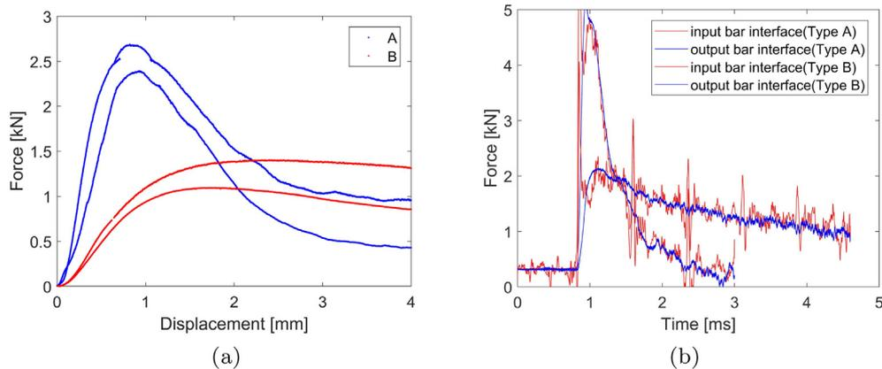
**Fig. 9.** Typical envelopes of the response curves (a) and specimen equilibrium check at interfaces between the transmitted and the input-reflected resultant wave during a split Hopkinson bar test (b) for air dried Type A and Type B.
