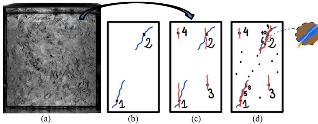
**Fig. 16.** Specimen (a) and schematic meso-scale representation of micro-flaws numbered in descending order of entity and crack paths, in blue lines for statics (b) and in red in dynamics for low (c) and high (d) number and density of flow distribution, with zoom on possible clay floccules separated by fibers.
