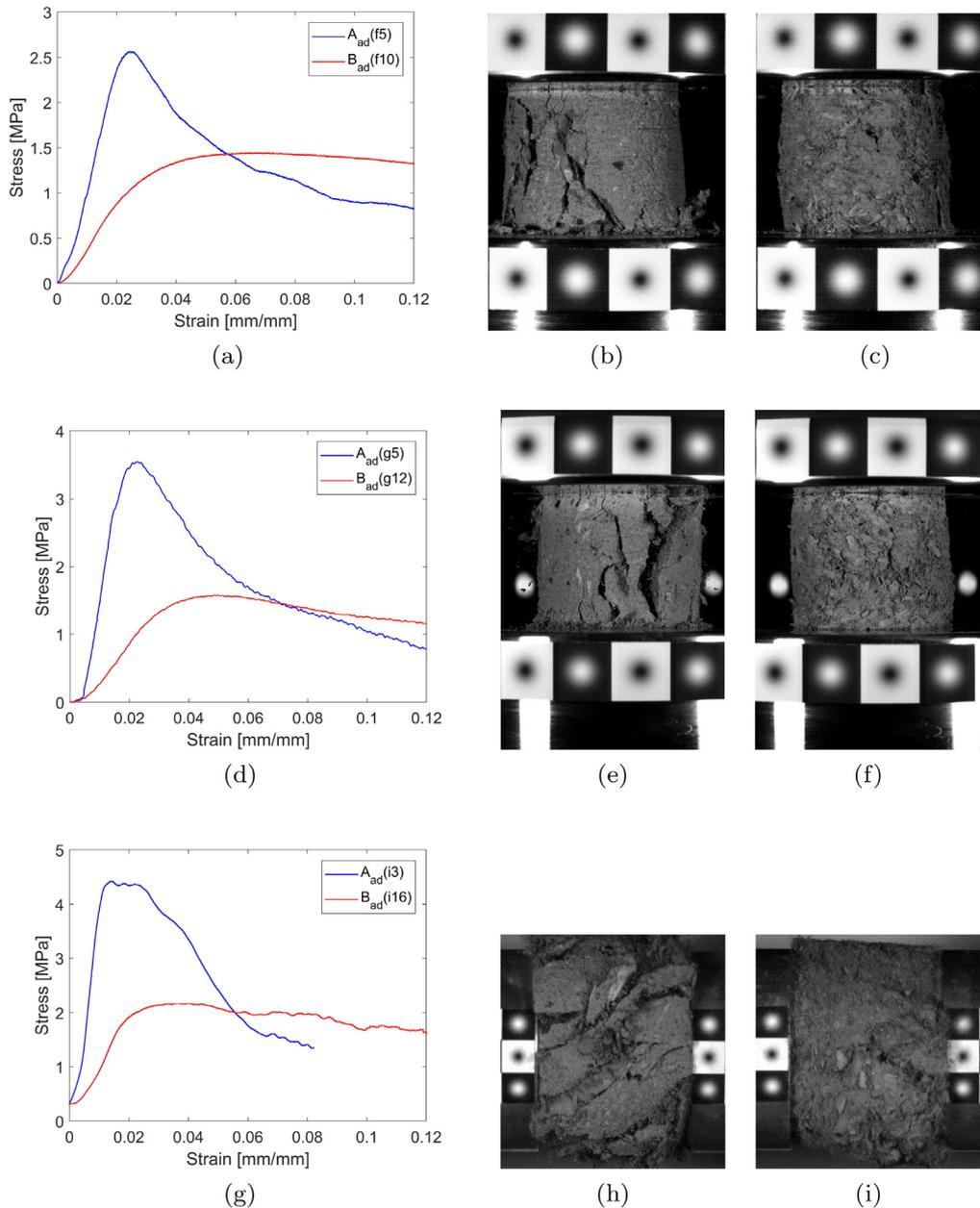
**Fig. 6.** Examples of stress strain plots and corresponding cracking patterns at 12% deformation for air dried Type A (left) and Type B (right) for static test (first row), intermediate strain rate test (second row) and split Hopkinson bar test (third row).
