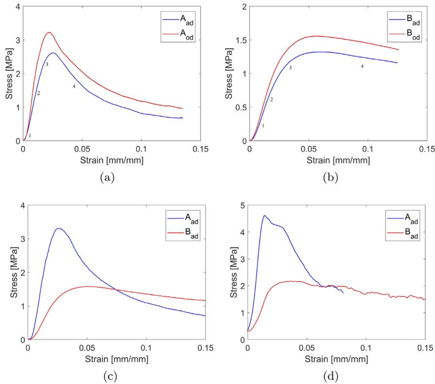
**Fig. 8.** Average normalized stress-strain plots for Type A and Type B in statics for both drying conditions (a, b) and in dynamics at intermediate strain rates (c) and split Hopkinson bar tests (d) for air dried condition.
