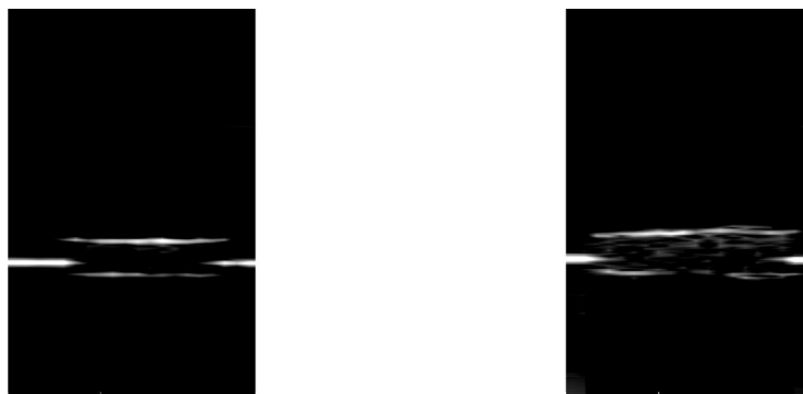
Fig. F.1. OCT images obtained for the analysis of the width of the PC 1-layer printed with the standard (left) and the optimized (right) nozzles at 5 mm 3 /s.
