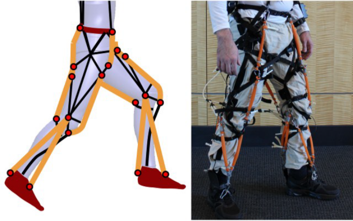
Figure 1.2: Image of the exosuit designed by Wehner et al. in 2013. The left picture shows the webbing in black. Each of the McKibben actuators, depicted in orange, is connected to a virtual anchor point, which are depicted with red dots. The right picture shows the real world application of the soft exosuit.
