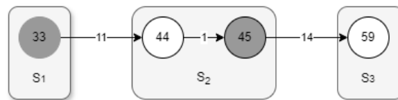
Figure 5.2: Event-activity network of a train service with a train service shift of 3 minutes.
