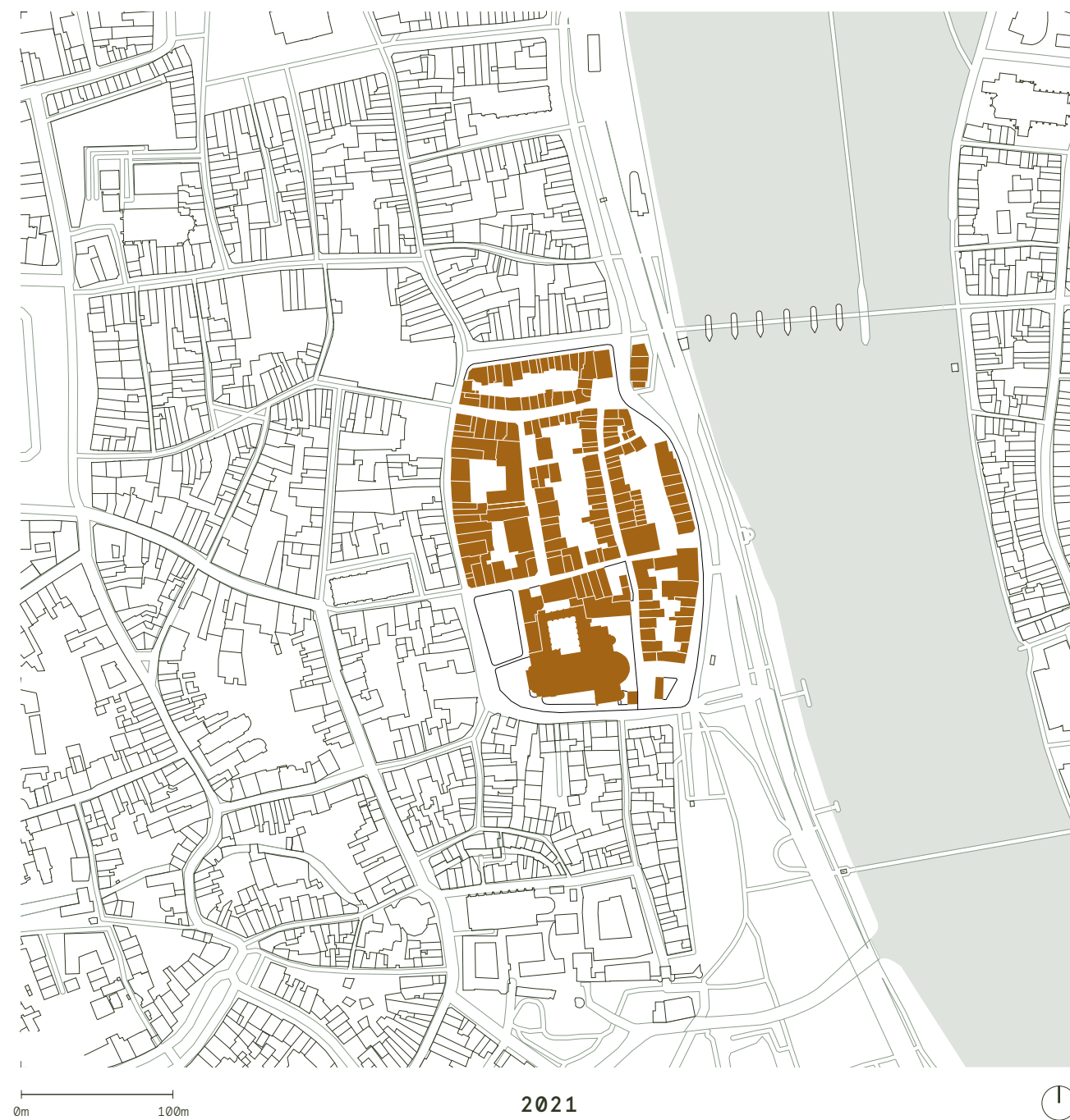
Insides of the blocks are 'carved out', by demolishing the backs of houses whilst preserving the front facades, bringing light and open space to the interior.
