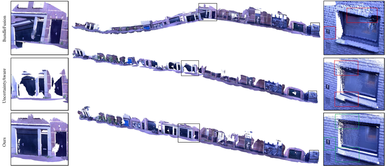
Fig. 20. Comparison of our reconstruction result (bottom row) with state-of-the-art RGB-D reconstruction systems, i.e., BundleFusion [Dai et al. 2017] (top row) and UncertaintyAware [Cao et al. 2018] (center row) on a sequence of 14,163 RGB-D frames captured on an urban street with a long trajectory. Closer inspections (black boxes) are presented to show the reconstructed details of each method.
