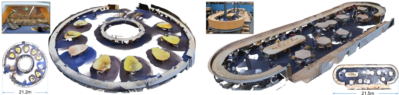
Fig. 1. Reconstruction of two large indoor scenes: (left) a study room of a university library and (right) a study platform in a grand hall of an academic building. The original two sequences consist of 16,128 (library) and 10,930 (study platform) RGB-D image frames, and the reconstructed model consists of 7,488,867 (library) and 7,904,727 (study platform) points, respectively. The average processing speed of our approach is around 43ms per frame, which demonstrates a nearly real-time performance. RGB-D data in these two experiments are captured by a Microsoft Kinect v1 sensor with a resolution of 640 \times 480 . Progressive results of the reconstruction can be found in the supplementary video.
