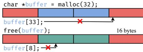
**Figure 2.** Example of a heap allocation protected by MTE. After allocation, the pointer and allocation are tagged with ■, while the surrounding memory is tagged with ■. When accessing memory, the hardware catches out-of-bounds errors (■ ≠ ■). When freeing memory, the memory region is retagged with ■. This prevents use-after-free errors (■ ≠ ■).
