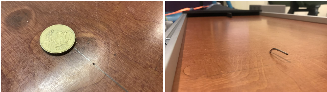
(a) Single static pressure tap (50 cent for reference).
