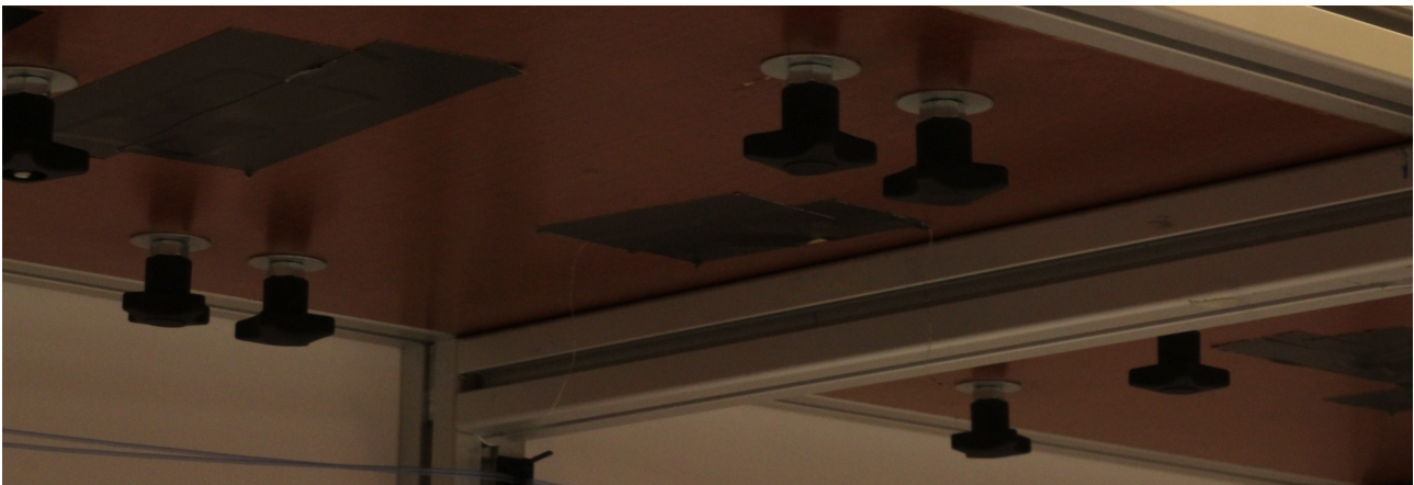
Figure F.7: Knobs that hold the test plate in place when underpressures are active.
