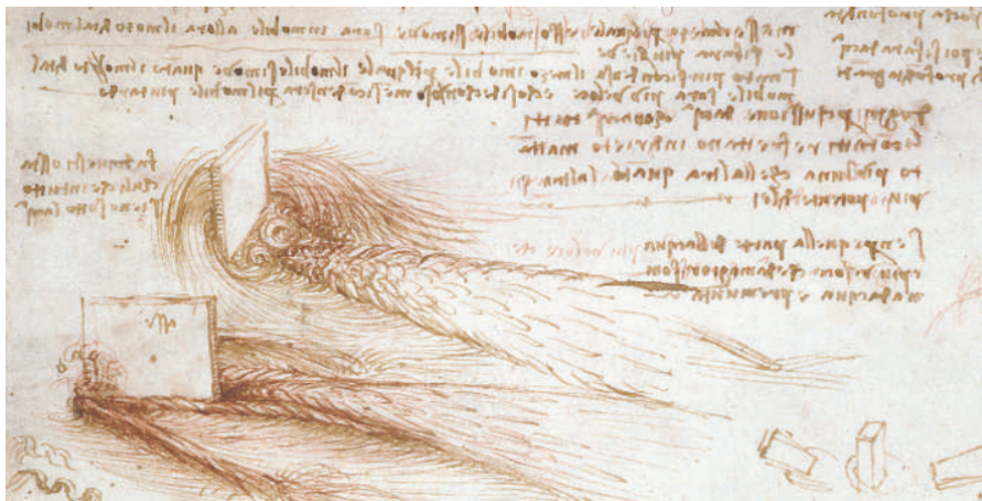
Figure 1.1: Sketches by Leonardo Da Vinci of flow fields over objects in a flowing stream (Da Vinci, 1509).
