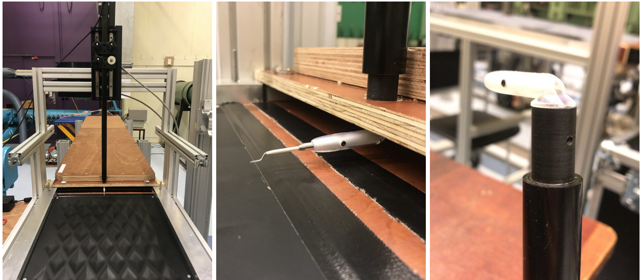
(a) Traverse with hollow rod. Flow from bottom to top. (b) Hotwire setup far away from the wall. Flow fltr. (c) Hollow rod with 3D printed probe support holder.
