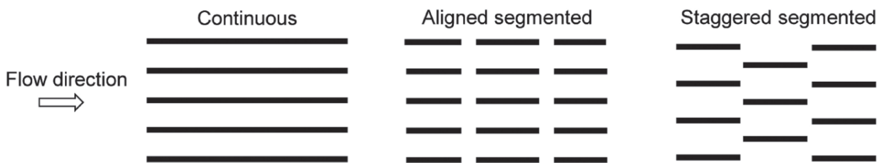
Figure 3.4: Different riblet configurations (Bixler and Bhushan, 2013a).
