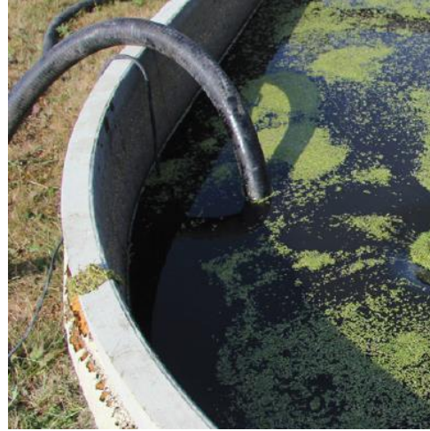
Figure 4.2e and f. Aquatic weed skimmer, featuring the onshore filtration unit and hoses (Meers and Coudron, 2018).
