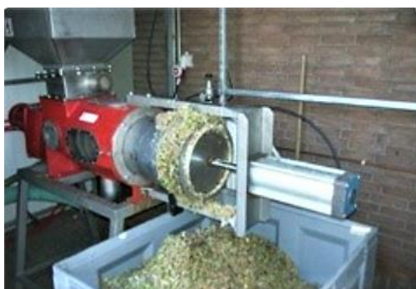
Figure 4.3a. Screw press Azolla treatment and b. ensilage treatment (Hoving et al., 2011).
