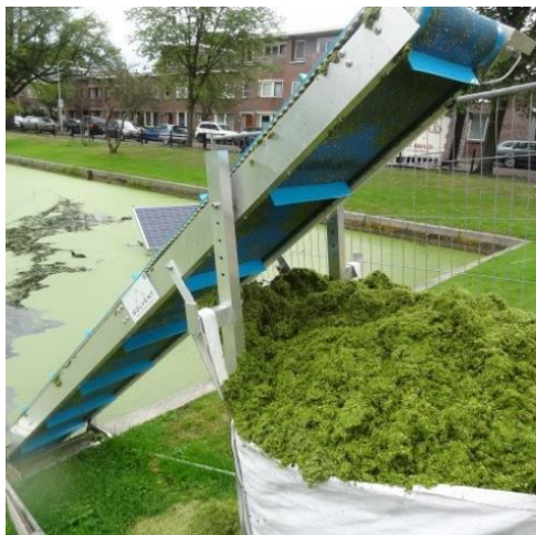
Figure 4.2c. and 4.2d. Solar-powered conveyor belt and aquatic weed brace (BomTechniek BV, n.d.).
