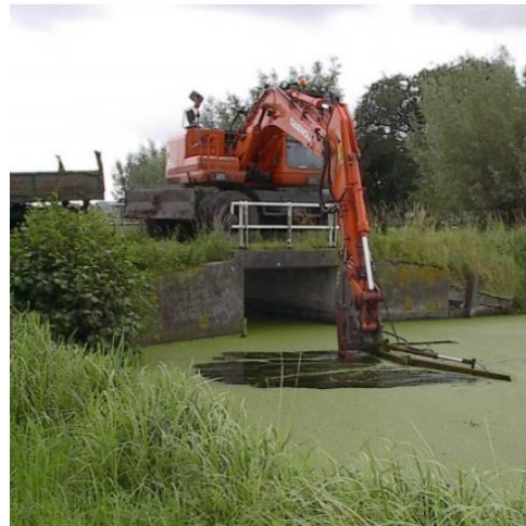
Figure 4.2a. and 4.2b. Wheeled excavator with dredge and wheeled excavator with flat sieve (Timmerman and Hoving, 2016).
