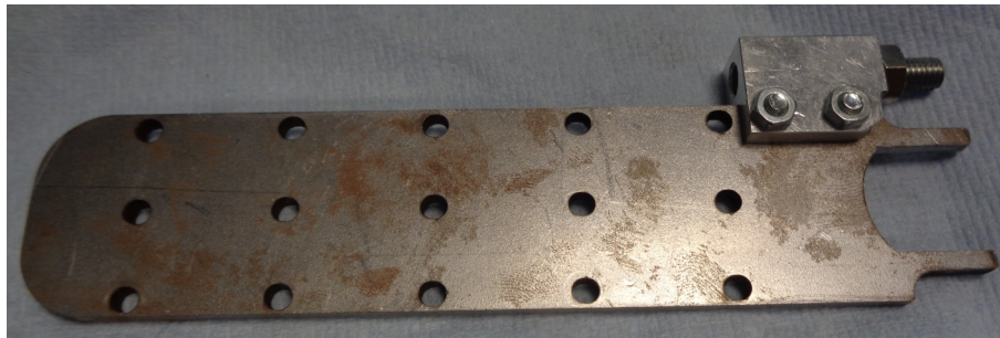
Figure G.4: Tension tool. This tool functions similar to a wrench. The set screw functions as adjustable reference.
