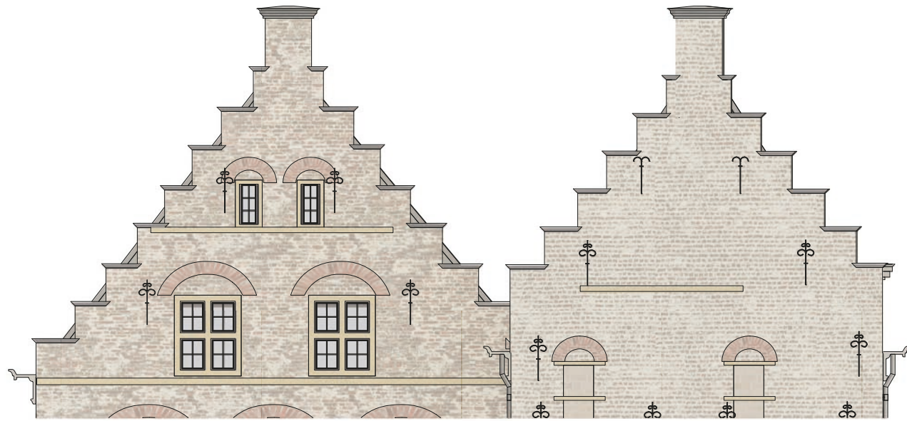
Front view gutter stepped gable façade
