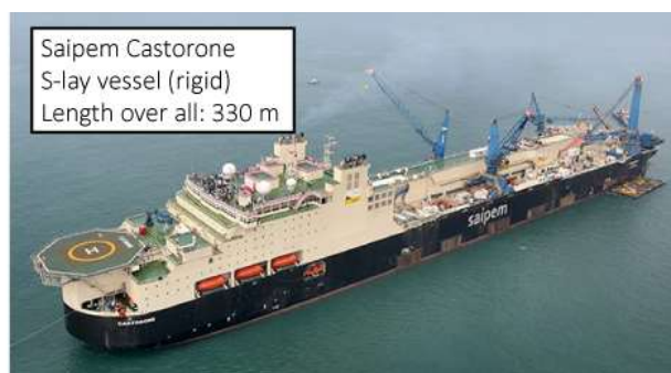
Figure A.2. The Lewek Constellation and the Saipem Castorone are two of the largest pipelaying vessels today. Both vessels can be resupplied with new pipes at sea (Images from: [27] [28])
