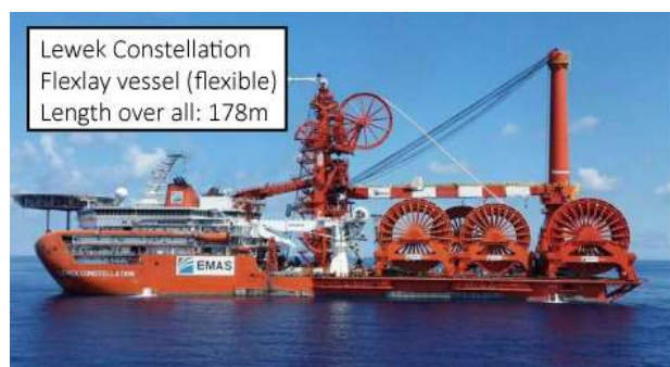
Figure A.2. The Lewek Constellation and the Saipem Castorone are two of the largest pipelaying vessels today. Both vessels can be resupplied with new pipes at sea (Images from: [27] [28])
