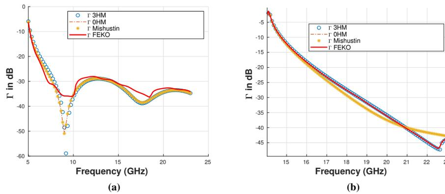
**Figure 3.** (a) Reflection coefficient for fundamental mode  $TE_{11}$  mode excitation inside the waveguide (b) Reflection coefficient for  $TE_{12}$  mode excitation inside the waveguide.
