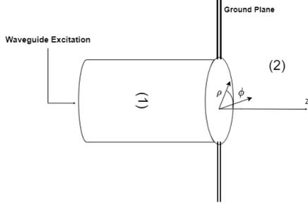
**Figure 1.** Geometry of cylindrical waveguide to free-space transition
