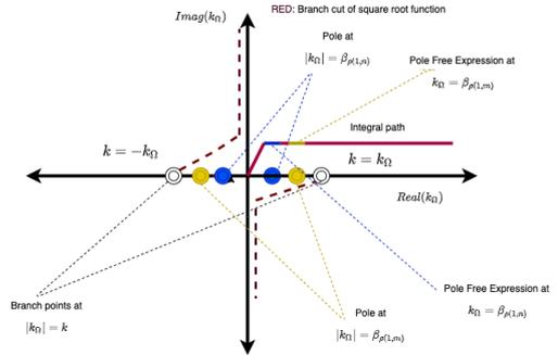
**Figure 2.** Integration path, branch cuts, branch points and poles to integrate K space integral
