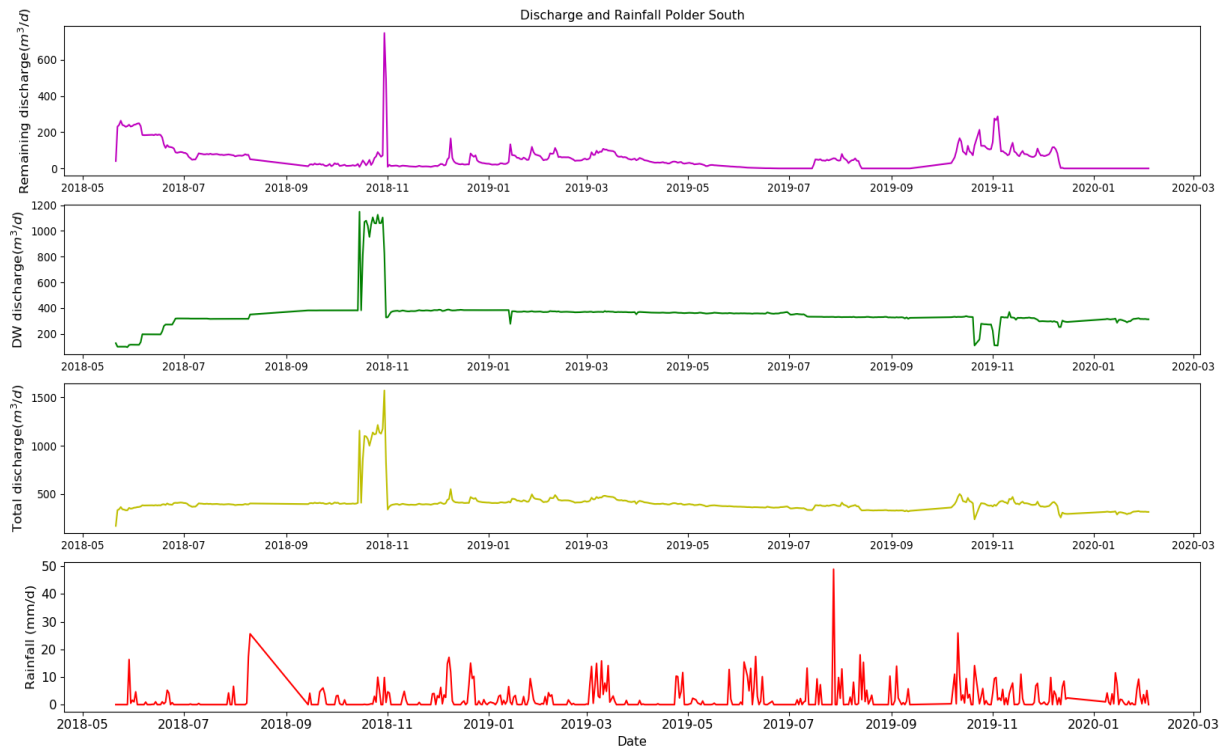
Figure 5.16: Overview of the discharge for Southern polder and the rainfall
