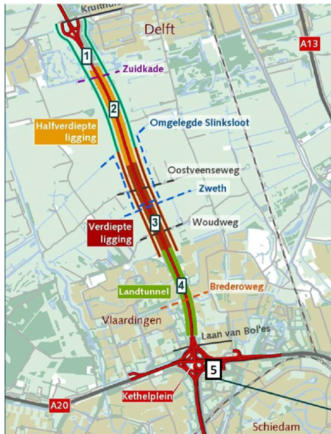
Figure 4.9: Location of the semi-sunken (halfverdiepte ligging) and sunken part (verdiepte ligging) of the motorway A4 Delft - Schiedam
