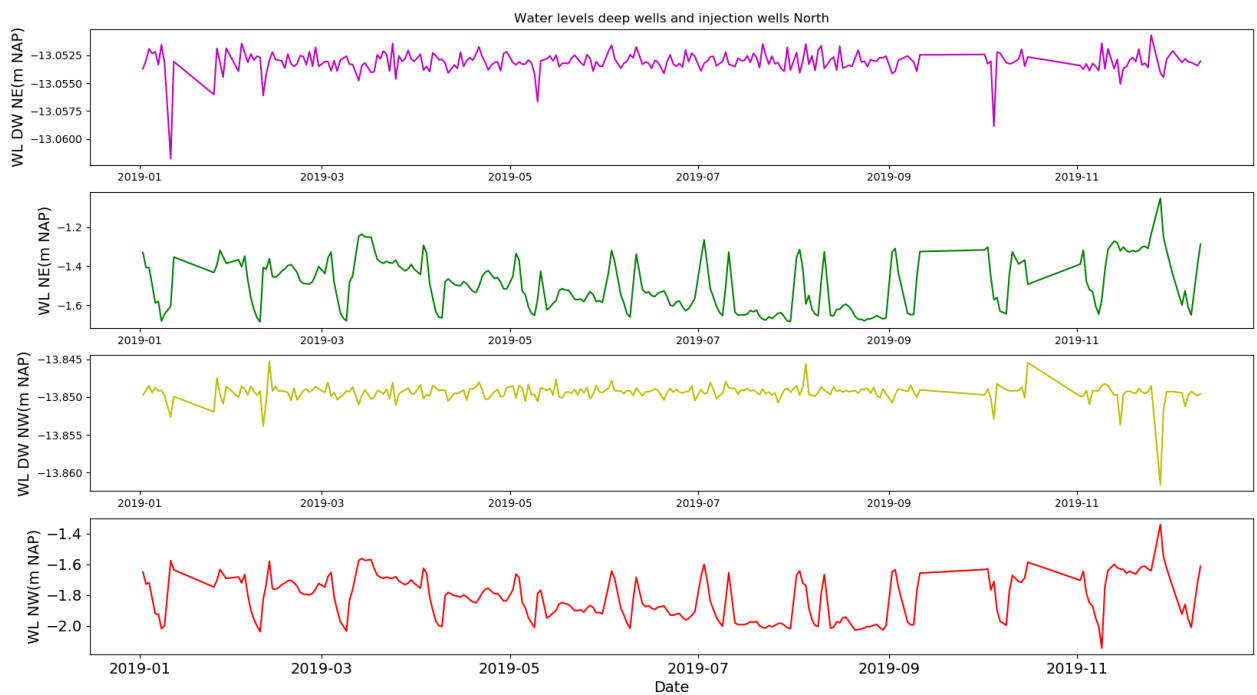
Figure 5.18: Overview of water levels in the deep wells and injection wells (Northern polder)
