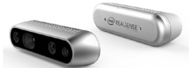
Fig.44: Intel's RealSense uses a combination of camera's and an infra-red grid projection to capture a 3D image. The compact design (20 x 6 cm) proves how small these camera's can be.
