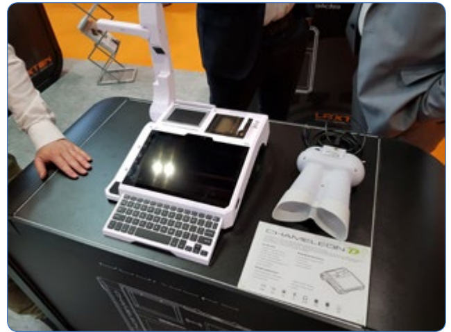
Fig.47: Chameleon-D, example of a compact portable identity enrolment device
