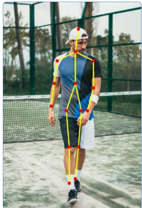
Fig.42: Parts of the body are identified through human pose estimation.
