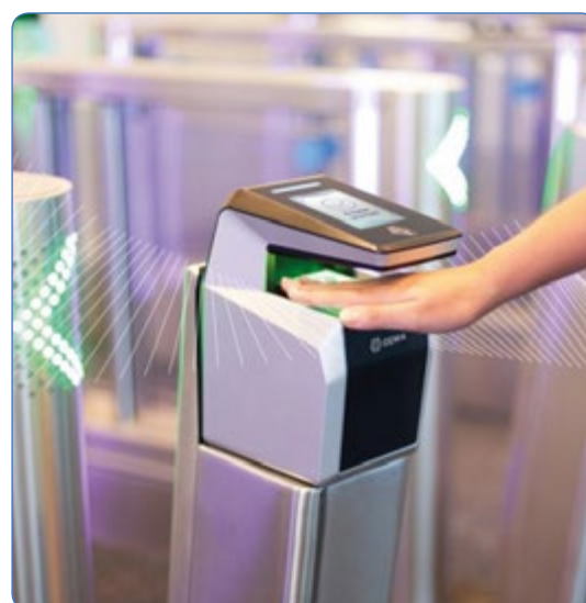
Fig.40: An example of touchless fingerprint scanning: Morpho-wave by Idemia.
