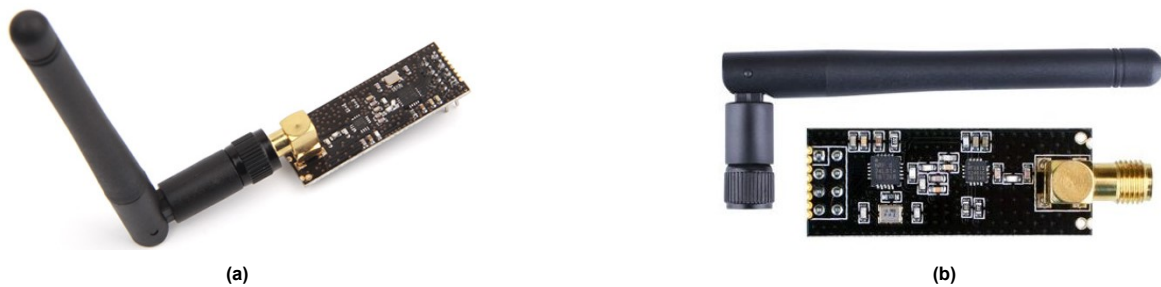
Figure 5.2: nRF24L01+ module with duck antenna: (a) assembled, and (b) disassembled.
