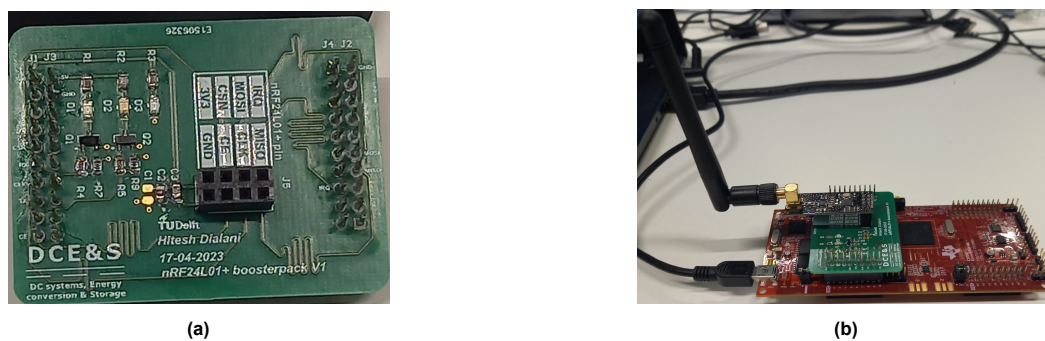
Figure 5.25: Assembled PCB: (a) nRF24L01+ boosterpack, and (b) nRF24L01+ boosterpack with nRF24L01+ and LaunchXL TMS320F28379D microcontroller stacked.
