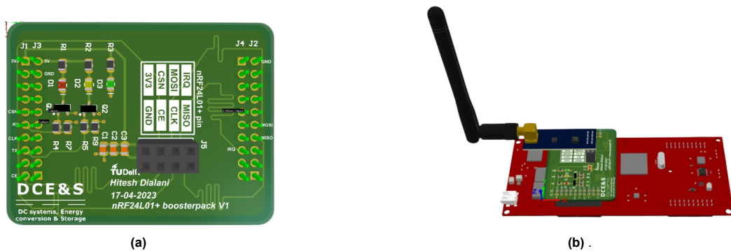
Figure 5.24: Altium PCB design showcasing: (a) the custom nRF24L01+ boosterpack, and (b) nRF24L01+ boosterpack with nRF24L01+ and LaunchXL TMS320F28379D stacked.
