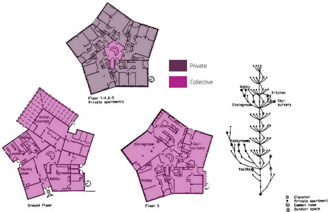
Fig. 7.5: 'Stacken', Sweden; typical floor plans + graph of 'tree-like' layout of the transition zone (Lindén, 1992) (coloured analysis by author)
