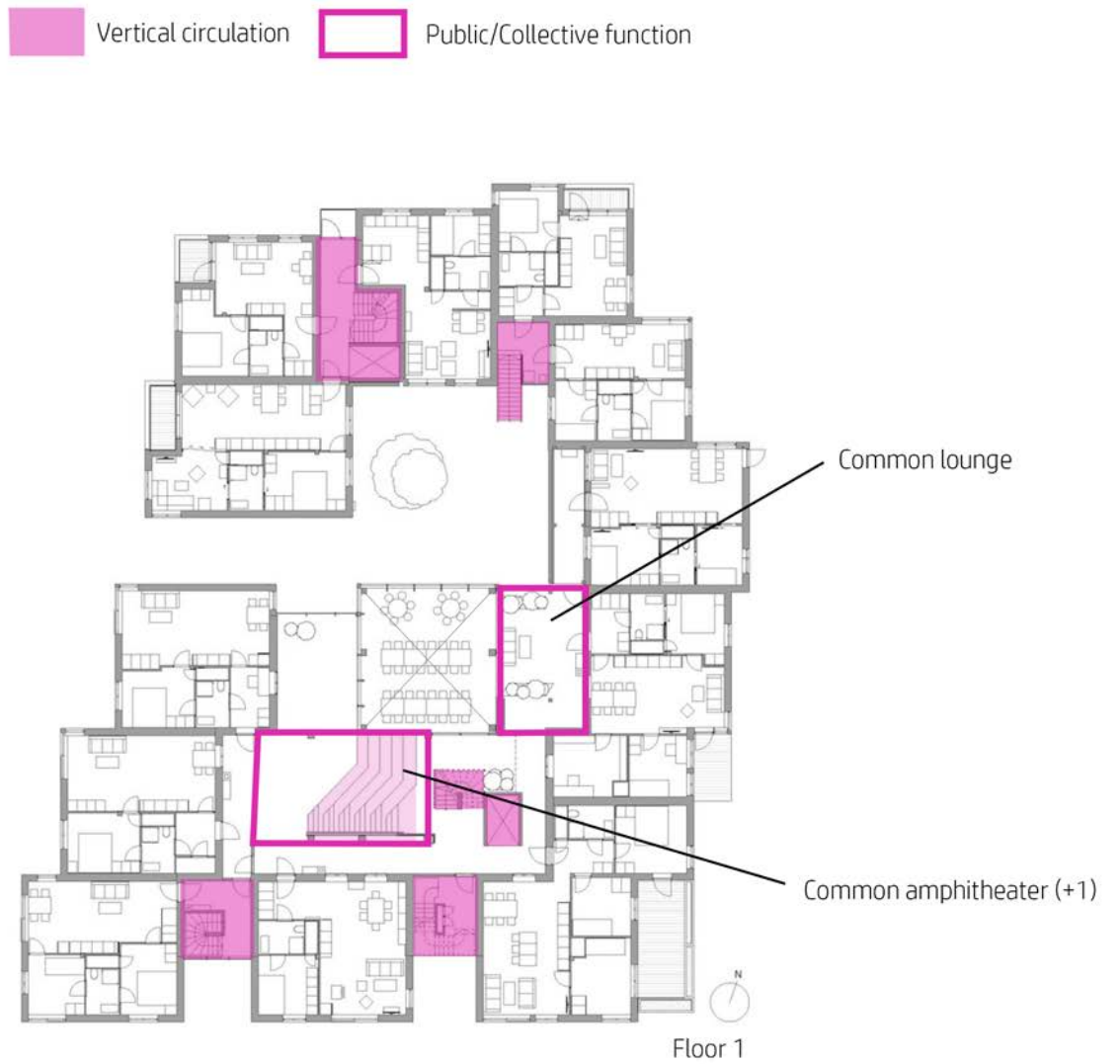
Fig. 7.32: Public/collective functions + vertical circulation; floor 1 (drawing by Helen&Hard Architects, 2019, and analysis + legend by author)
