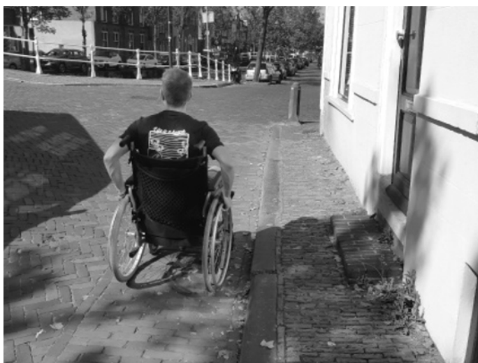
Fig. 2.5 (by author): ‘Obstacles on small pavements like a stepping stone can force the wheelchair user to continue on the road, forming a danger for themselves and other road users like cyclists, scooters or cars. Especially in narrower streets this is a problem.’
