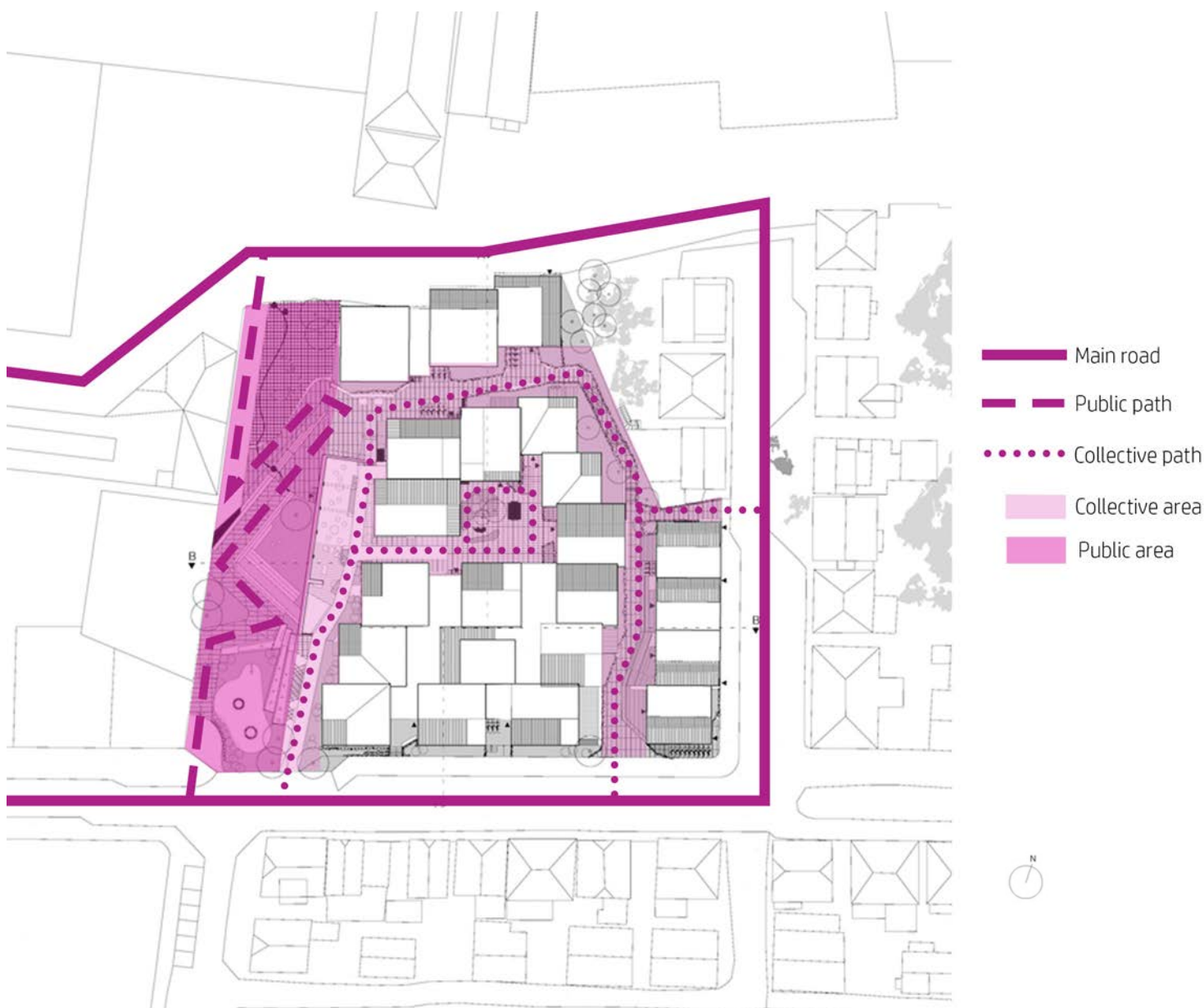
Fig. 7.25: Level of collectivity of the exterior spaces in the close vicinity of the project + hierarchy of the ways of mobility (paths, streets, etc.) (drawing by Helen&Hard Architects, 2019, and analysis + legend by author)
