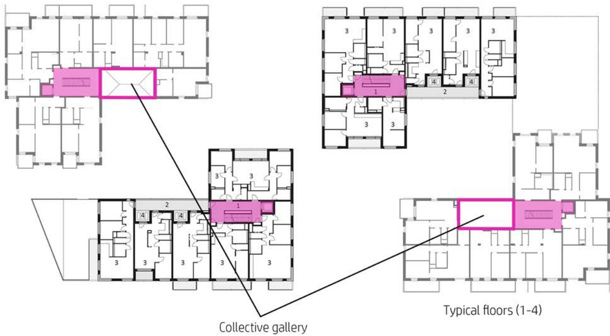
Fig. 7.60: Public/collective functions + vertical circulation; floor 1-4 + 5 (drawing by Trans_city Architects, 2018, and analysis + legend by author)
