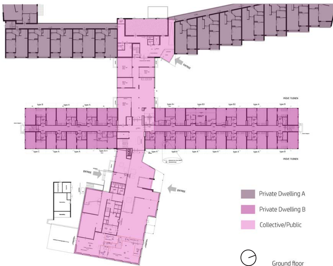
Fig. 2.21: Lay-out of Huis Assendorp, showing the two residential wings and the collective wing connecting everything (plan provided by Huis Assendorp, Zwolle; analysis by author)
