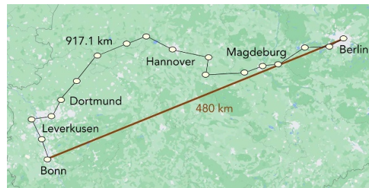
Figure 1. Map of Germany overlaid with a depiction of the fiber path connecting the German cities of Bonn and Berlin that we investigate, provided by Deutsche Telekom (DT). The white circles represent locations where DT plans to install trusted nodes and where, when building a repeater chain, processing nodes or heralding stations could be placed. These locations are connected to each other through fiber drawn in black. The maximum number of repeaters that can be placed between Bonn and Berlin in this fiber network is seven. We consider all possible repeater placements, assuming that the heralding stations are placed as symmetrically as possible (there are 986 such placements). The distance between Bonn and Berlin is 917.1 km via fiber, and approximately 480 km as the crow flies. The reason for such a large difference between the two values is that other major German cities, such as Hannover and Dortmund, are connected through the fiber link as well.
