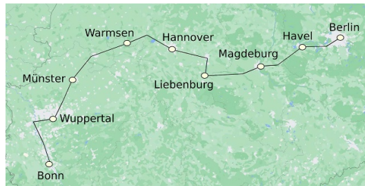
Figure 8. Map of Germany overlaid with a depiction of the fiber path connecting the German cities of Bonn and Berlin that we investigated. The white circles represent end nodes, in Bonn and Berlin, and repeater nodes elsewhere. This placement corresponds to the best found by our optimization method, in the sense that it allowed for minimization of hardware requirements for a target secret-key rate of 10 Hz.
