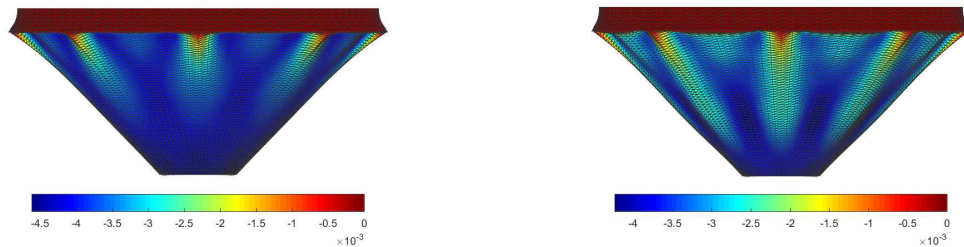
Figure 6.28: Displacement for a stiffened tapered thickness design for \Delta T = 0\text{K} , scale = 30. Left: Axial displacement displayed on the total deformed structure for the QI-design. Right: Axial displacement displayed on the total deformed structure for the VS-design.
