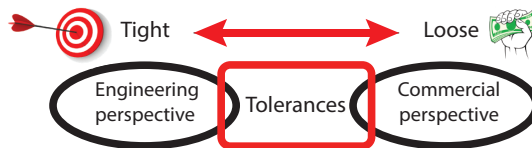
Figure 1.6: The quality dilemma when producing automotive turbochargers.
