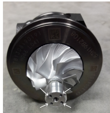
(b) Modified turbocharger rotor-bearing system: front view. Grub screws can be inserted in the holes indicated by the arrows.
