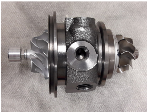
(a) Modified turbocharger rotor-bearing system: top view. The rotor features an additional cylindrical section in front of the compressor wheel (left hand side).
