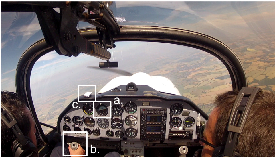
Figure 4.3: A screenshot of the video recording of the in-flight experiment. Left is the participant with the AI (a) the centerstick (b) and the IMU (c) visible, right is the test pilot.
