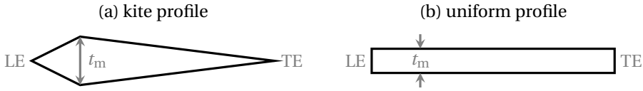
Figure 3.2: Schematic diagram of two cross-sectional profiles that are used to describe the chordwise mass distribution. The maximal thickness of the cross-section is denoted as t_m . LE and TE represent the leading edge and trailing edge, respectively.
