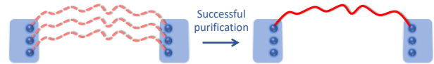
Fig. 1. Purification example. Two nodes, with three quantum memories each, begin with three imperfect entangled states (red curves, dashed). After purification is carried out (successfully in the example), the nodes are left with a higher-quality single entangled state (red curve, solid).
