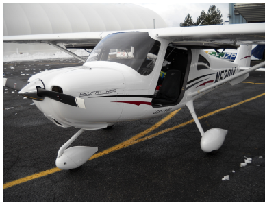
Figure 21.1: Door design Cessna Skycatcher [93]
