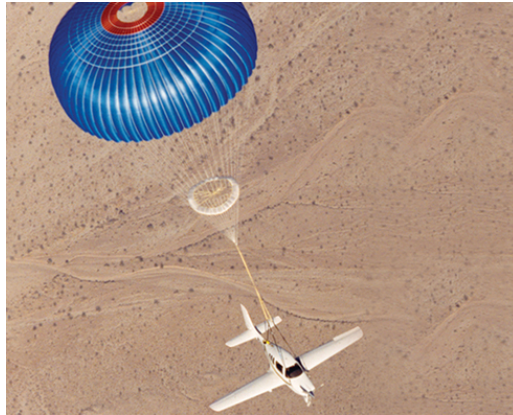
Figure 17.2: Picture of the parachute system of a Cirrus aircraft [58]
