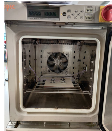
(a) Sensors in the climate chamber
