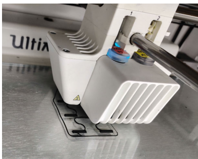
(a) The printing process for the sensors
