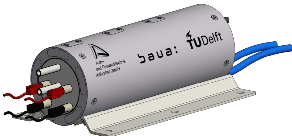
Figure 1.2: CAD-model of the nano-PMC. Depicted are the aluminium frame enclosing the classifier, inlet, outlet, electrical connections and water conduit for temperature control.
